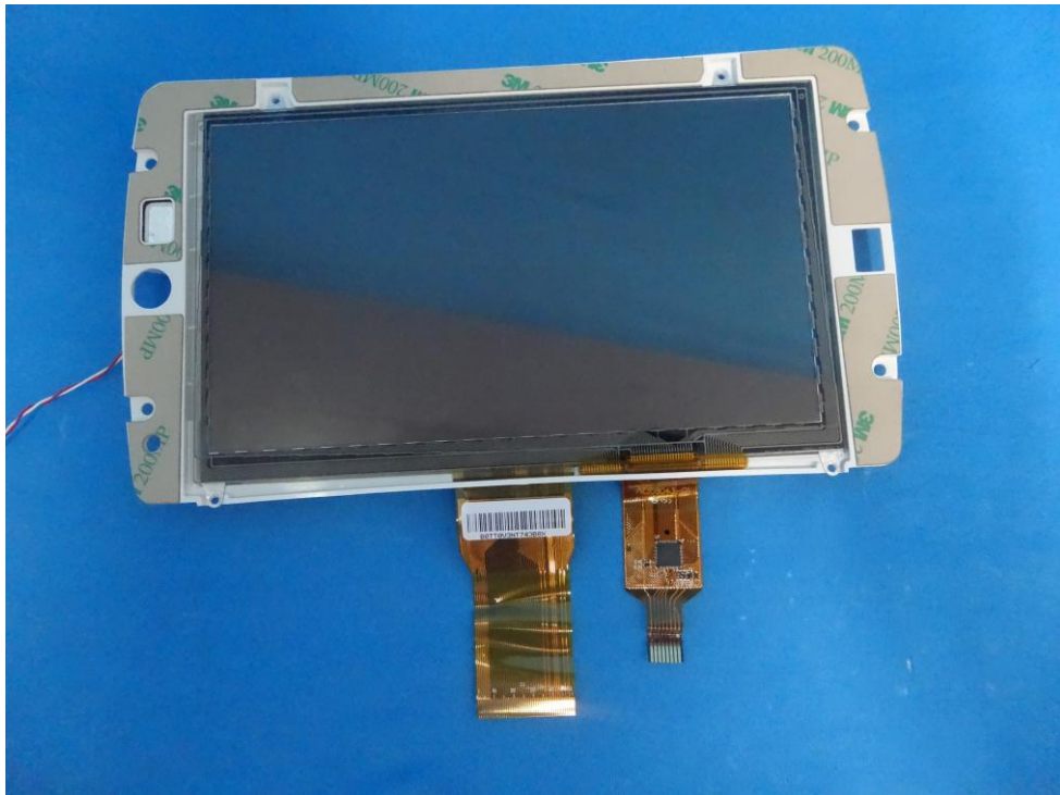
EUT Display Removed
