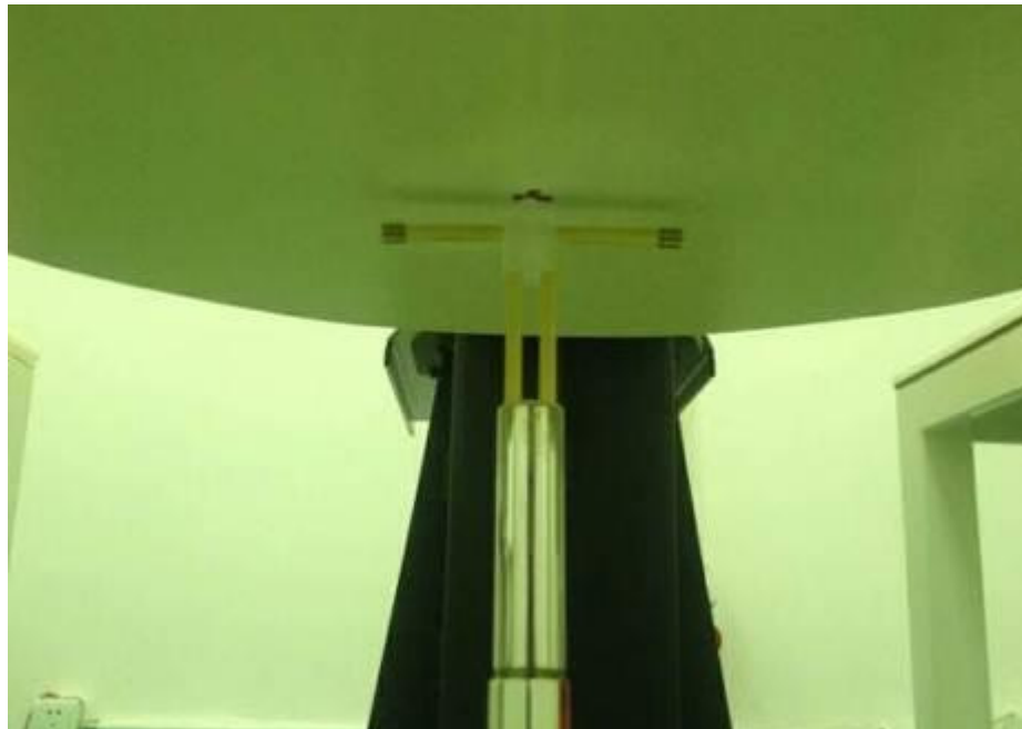
Picture 8.2 Photo of Dipole Setup
