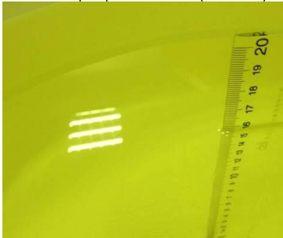
Picture 7-4 Liquid depth in the Flat Phantom (1800 MHz Body)
