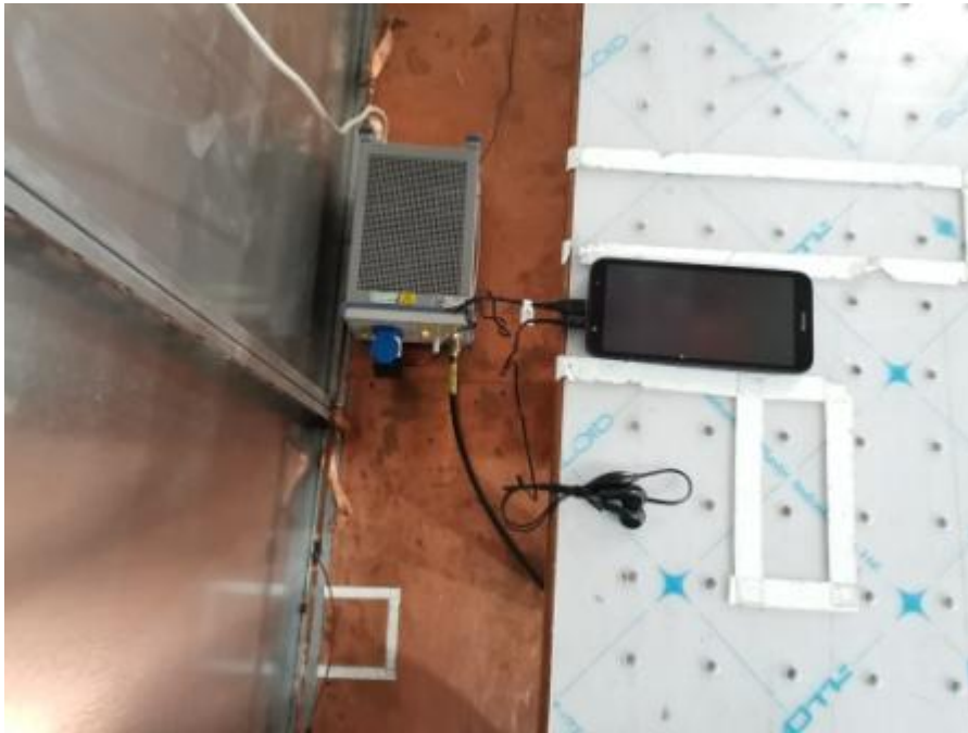
Conducted Emissions Test Setup (with charger)
