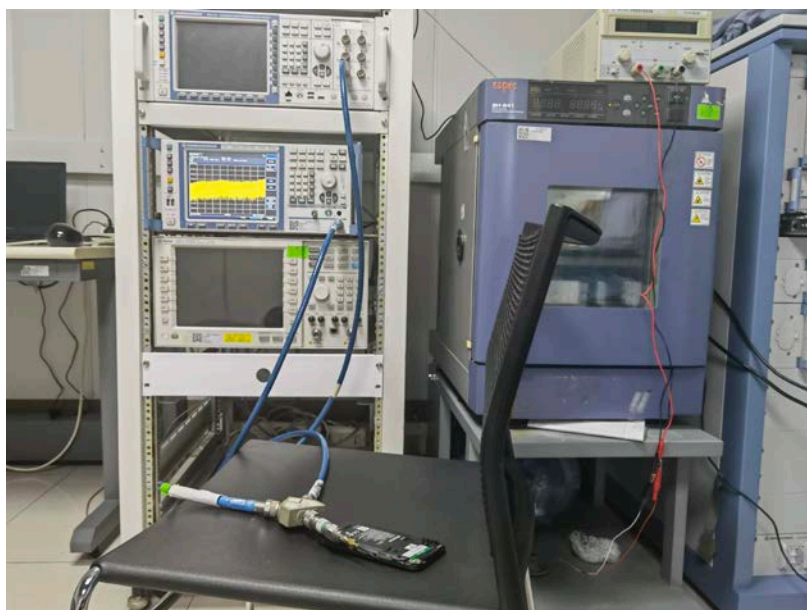
RF Conducted Test setup (GSM/WCDMA/LTE)
