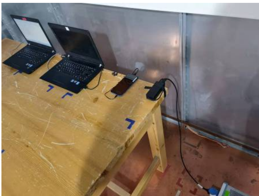
Conducted Emissions Test Setup (with laptop)
