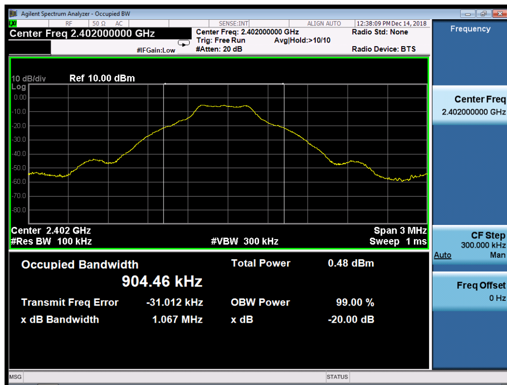
TEST PLOT OF BANDWIDTH FOR LOW CHANNEL
