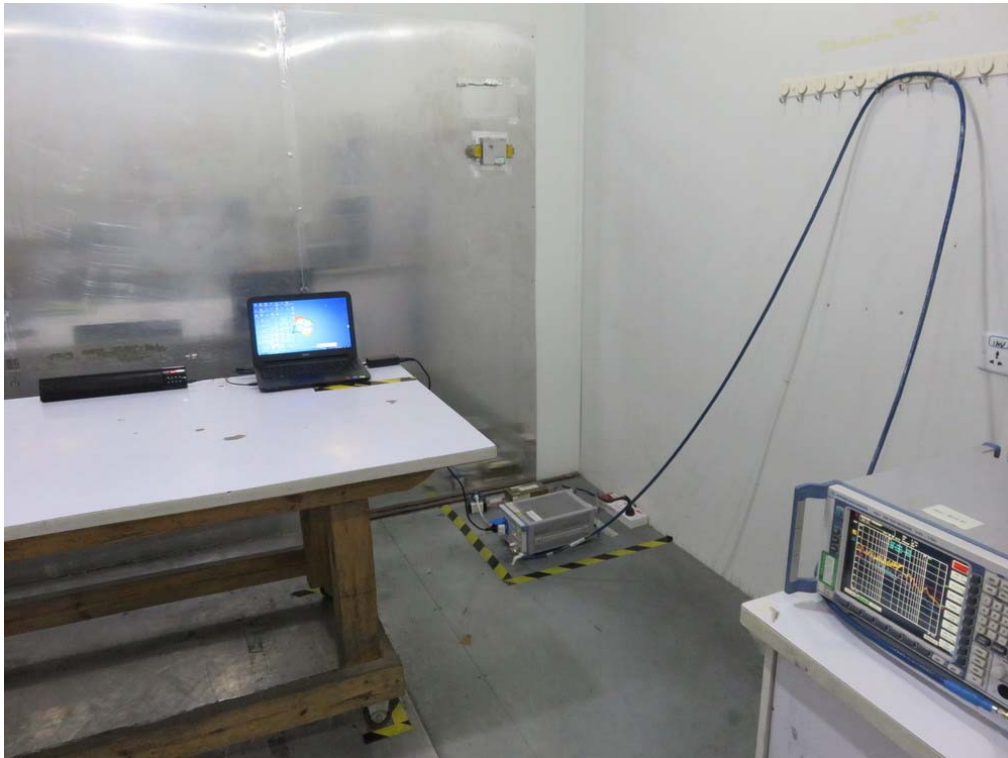
FCC RADIATED EMISSION TEST SETUP
