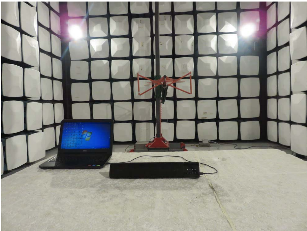
FCC RADIATED EMISSION TEST SETUP
