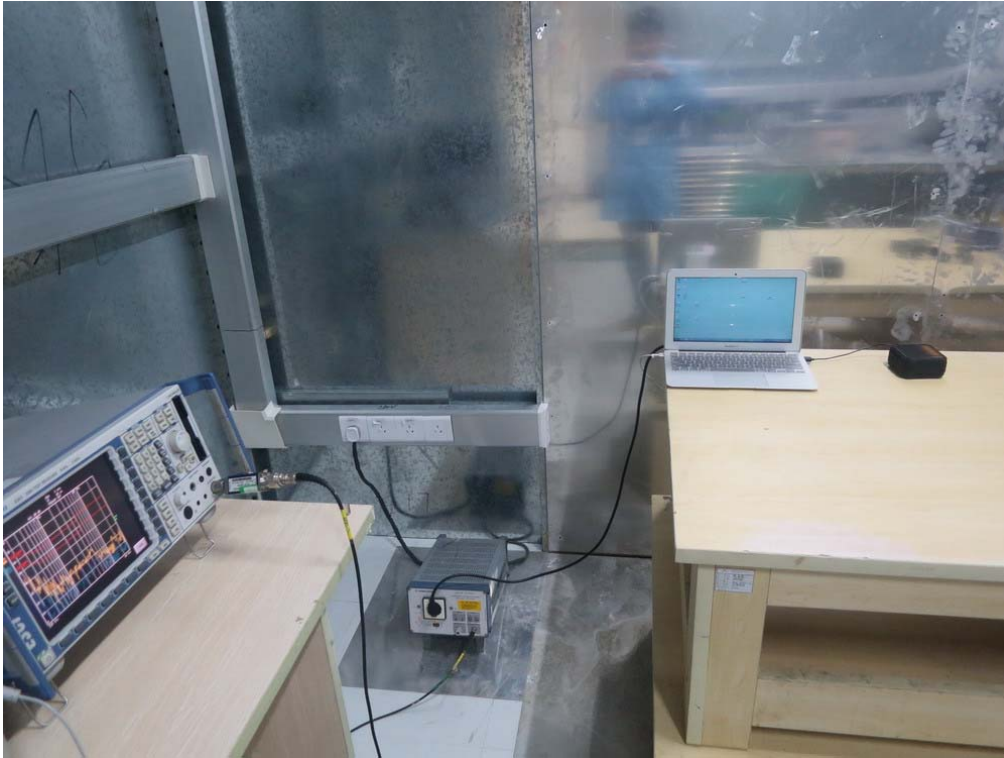
FCC RADIATED EMISSION TEST SETUP
