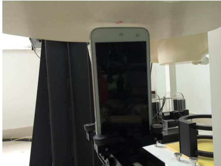
10mm Body-worn Bottom Side Setup Photo
