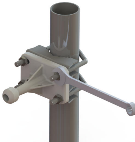
Figure 14: Tightening the 4 nuts
