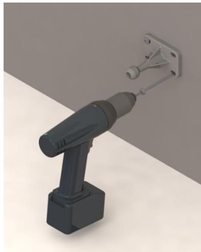
Figure 9: Screwing the mounting bracket
