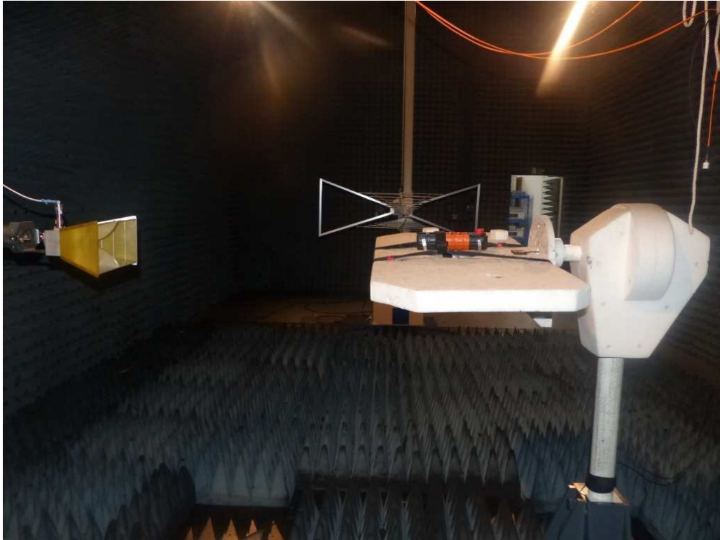
Photo 3: Test setup for radiated measurements (Enclosure, fully-anechoic chamber, above 1 GHz intentional radiator §15)
