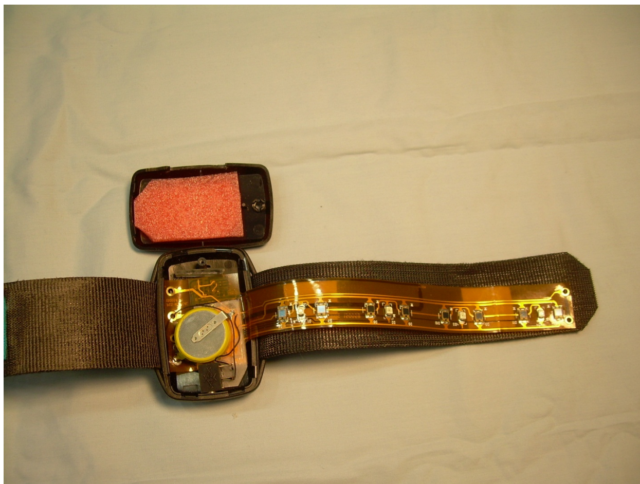
Photograph 7 – View with the XTMR 103 Housing Opened
