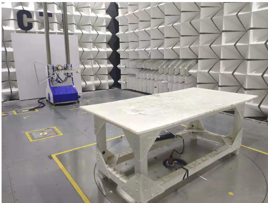
Radiated spurious emission Test Setup-1(Below 1GHz)
