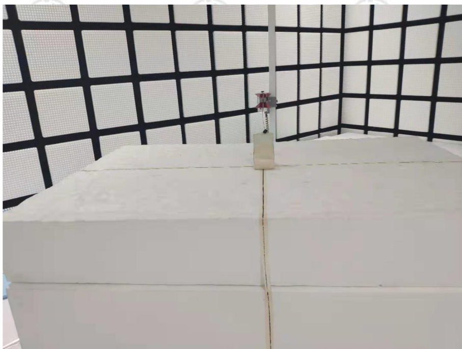
Radiated spurious emission Test Setup-2(Above 1GHz)
