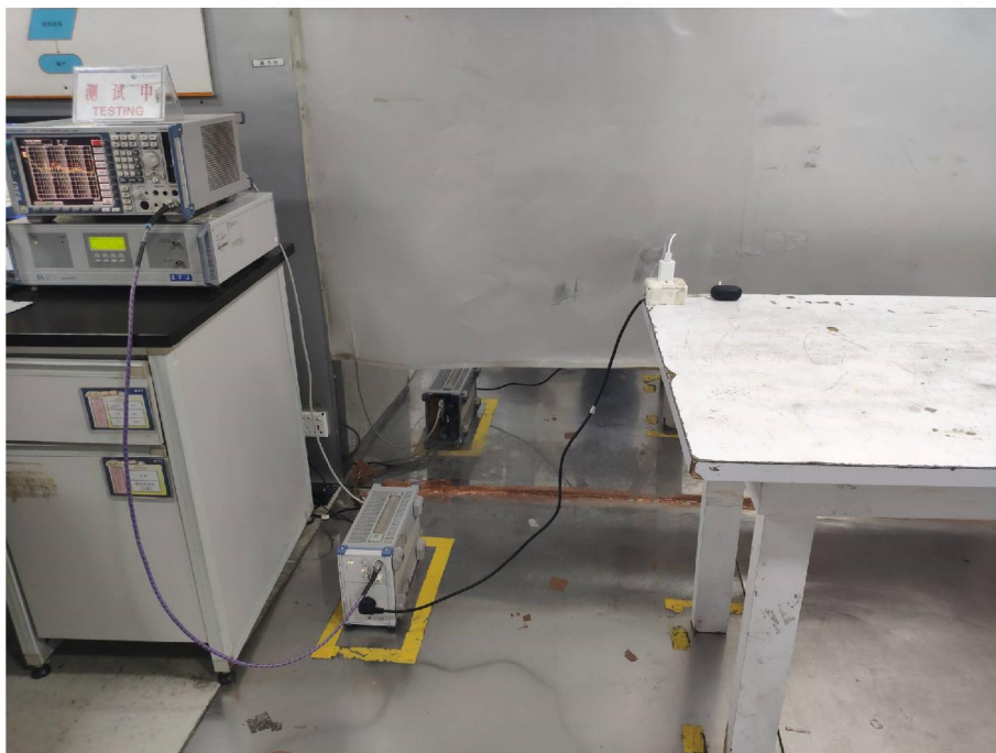
Conducted Emissions Test Setup
