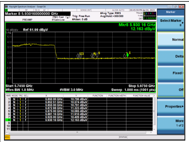
Middle channel Band edge (Peak) - Band 3
