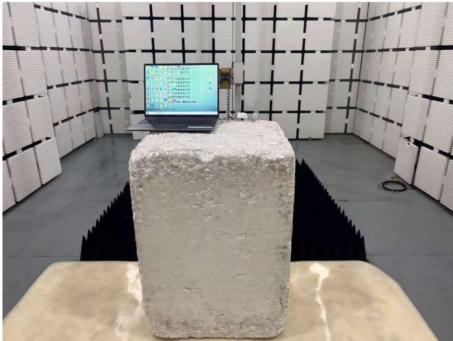
Set-up for Radiated Spurious Emission, Above 1GHz
