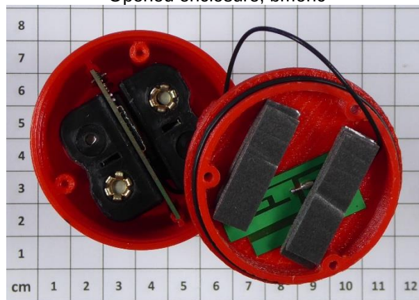
Opened enclosure, bmonc
