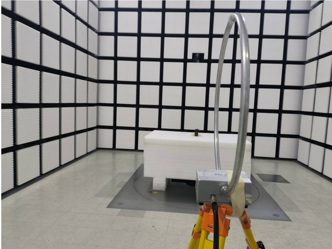
Radiated Emission Below 30MHz View Perpendicular
