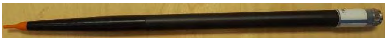
Figure 1 – MVG COMOSAR Dosimetric E field Probe
