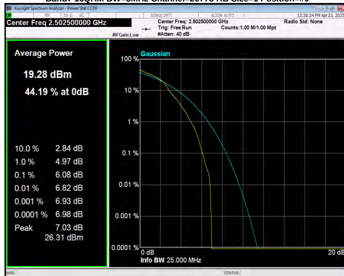
Band7 16QAM BW=5MHz Channel=21100 RB Size=1 Position=#0
