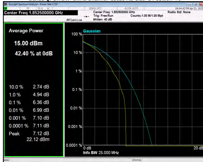
Band2 QPSK BW=5MHz Channel=18900 RB Size=1 Position=#0
