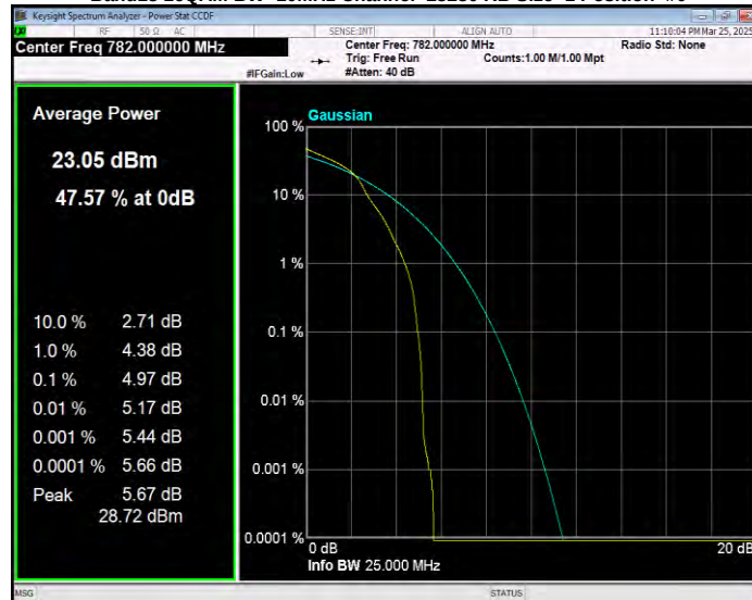
Band13 16QAM BW=5MHz Channel=23205 RB Size=1 Position=#0
