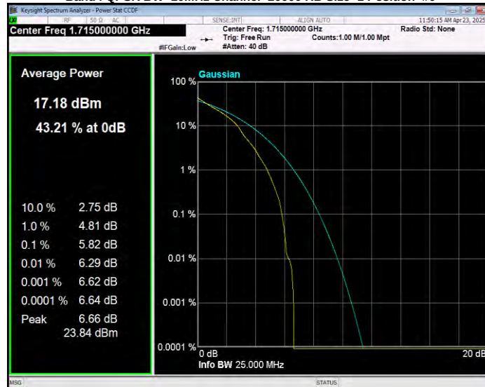
Band4 QPSK BW=10MHz Channel=20175 RB Size=1 Position=#0
