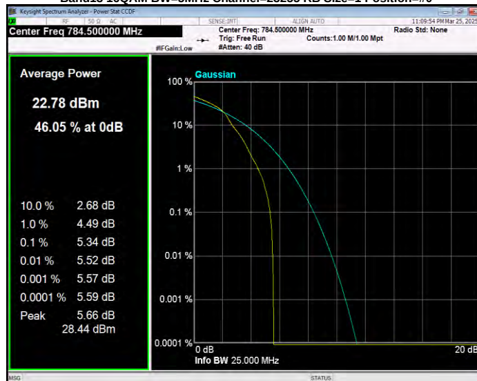
Band13 QPSK BW=10MHz Channel=23230 RB Size=1 Position=#0
