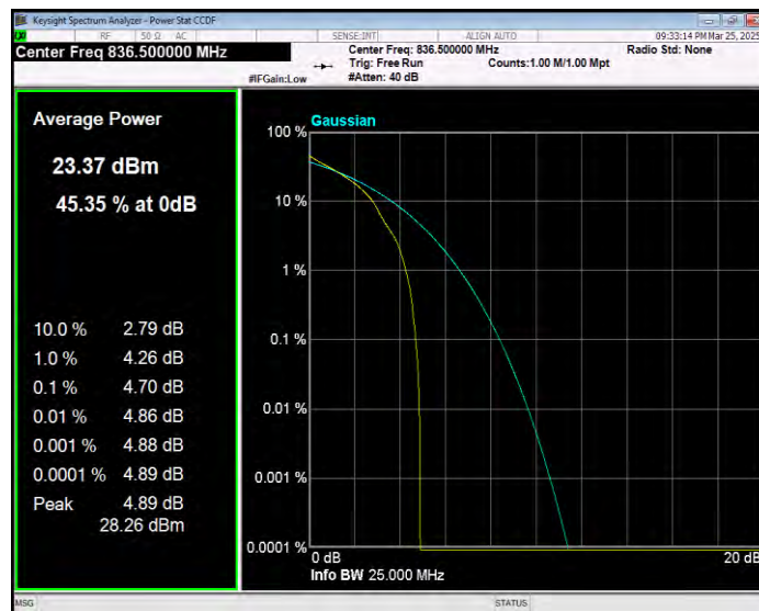
Band5 QPSK BW=3MHz Channel=20635 RB Size=1 Position=#0
