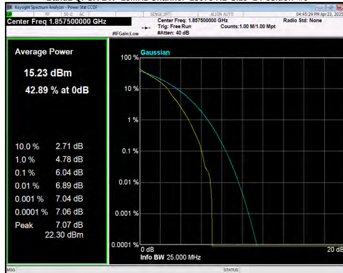
Band2 QPSK BW=15MHz Channel=18900 RB Size=1 Position=#0
