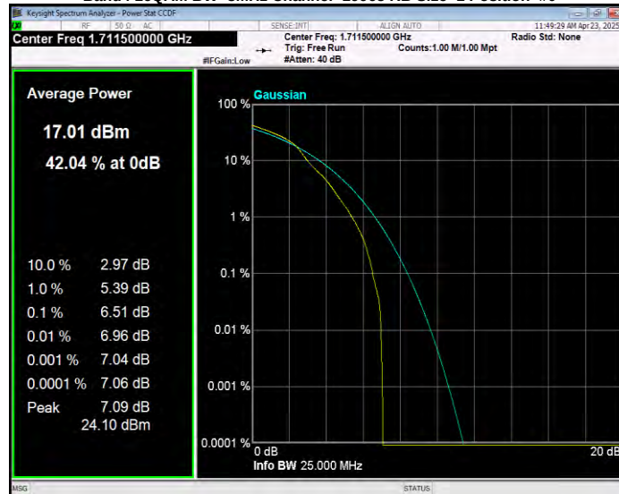
Band4 16QAM BW=3MHz Channel=20175 RB Size=1 Position=#0
