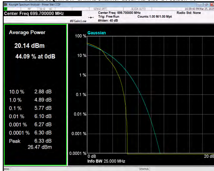
Band12 16QAM BW=1.4MHz Channel=23095 RB Size=1 Position=#0
