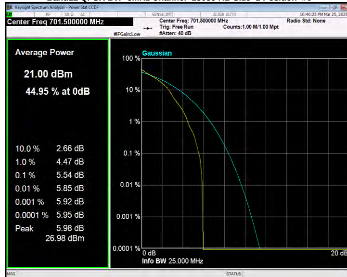
Band12 QPSK BW=5MHz Channel=23095 RB Size=1 Position=#0
