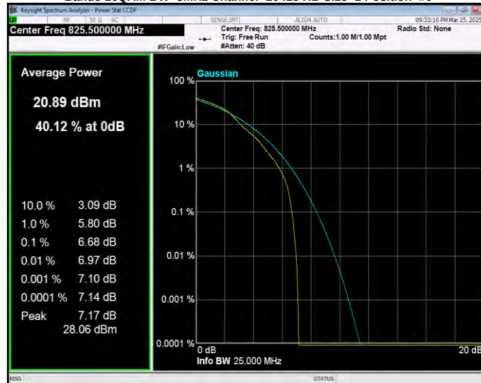
Band5 16QAM BW=3MHz Channel=20525 RB Size=1 Position=#0
