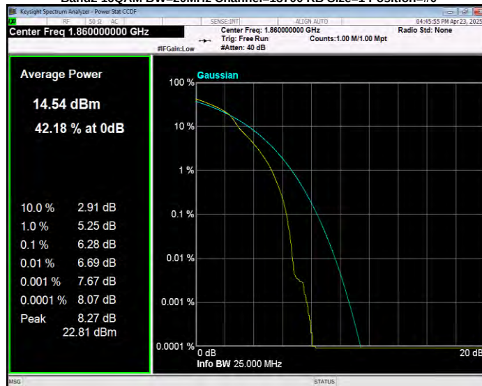
Band2 16QAM BW=20MHz Channel=18900 RB Size=1 Position=#0
