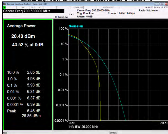
Band12 16QAM BW=3MHz Channel=23095 RB Size=1 Position=#0
