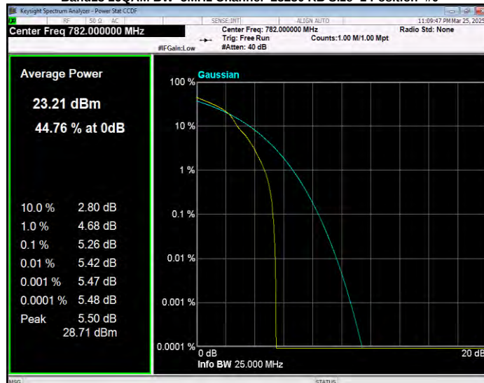
Band13 16QAM BW=5MHz Channel=23255 RB Size=1 Position=#0
