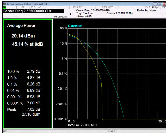
Band7 16QAM BW=15MHz Channel=21375 RB Size=1 Position=#0
