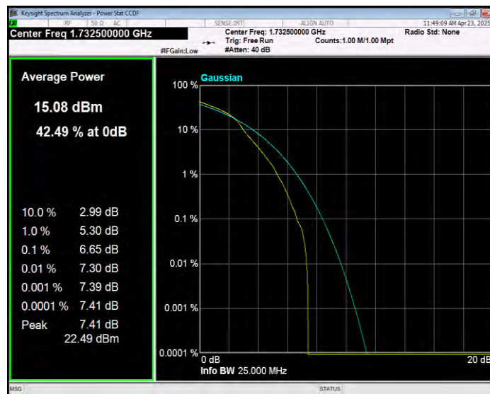
Band4 16QAM BW=1.4MHz Channel=20393 RB Size=1 Position=#0
