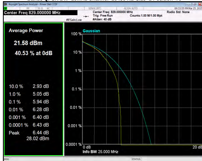
Band5 QPSK BW=10MHz Channel=20525 RB Size=1 Position=#0
