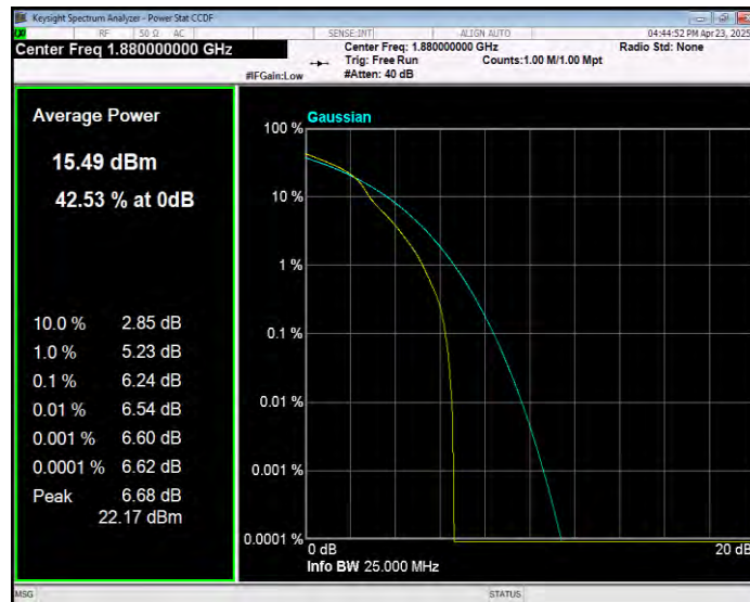
Band2 16QAM BW=5MHz Channel=19175 RB Size=1 Position=#0
