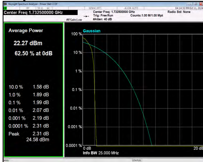
Band4 QPSK BW=10MHz Channel=20350 RB Size=1 Position=#0
