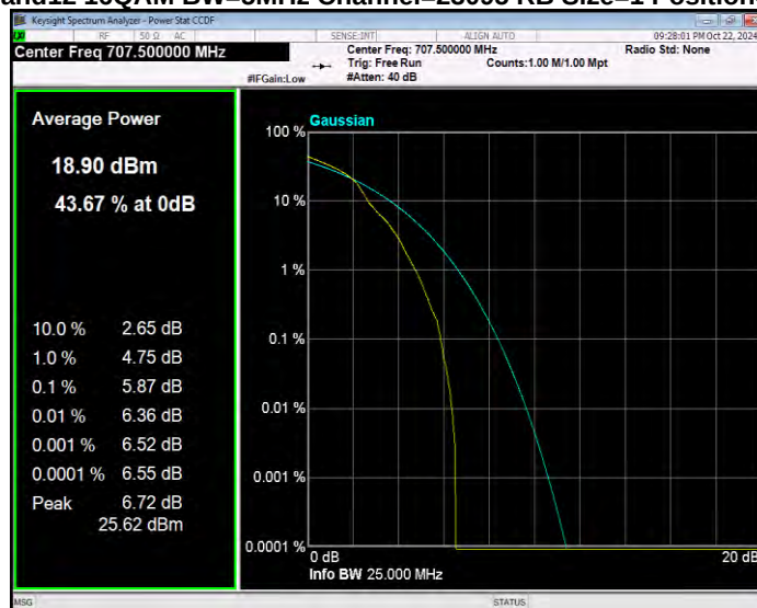
Band12 16QAM BW=5MHz Channel=23155 RB Size=1 Position=#0
