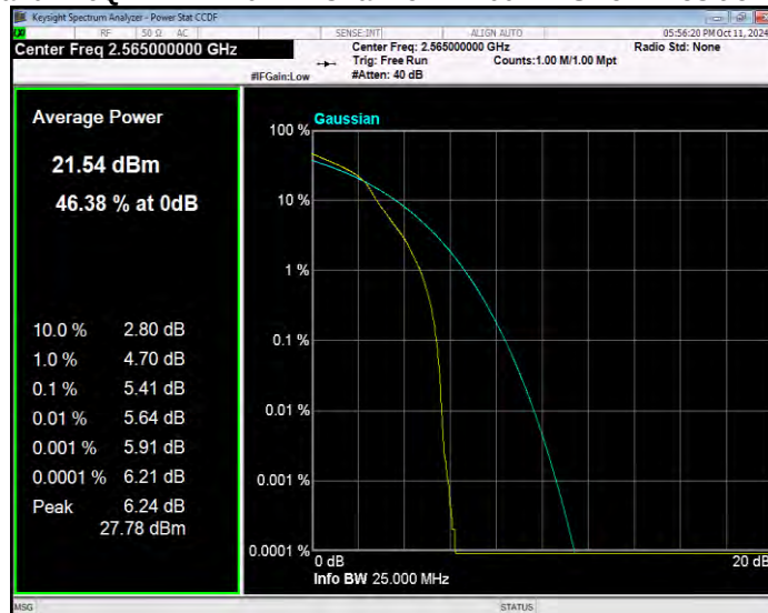
Band7 16QAM BW=15MHz Channel=20825 RB Size=1 Position=#0
