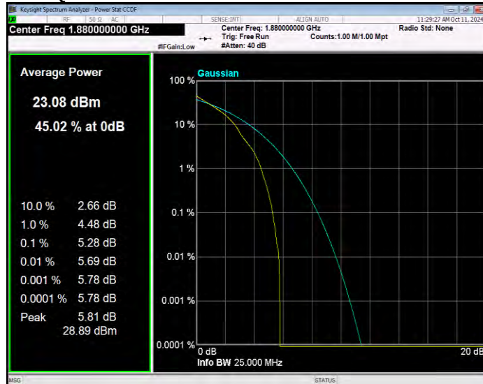
Band2 QPSK BW=3MHz Channel=19185 RB Size=1 Position=#0
