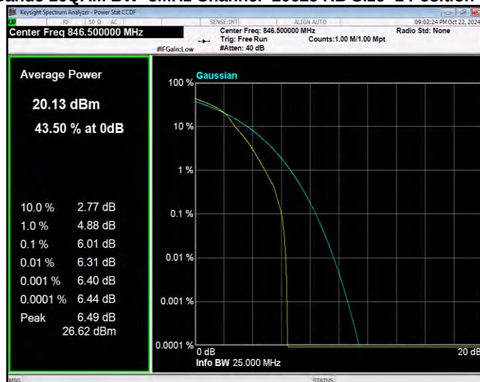
Band5 QPSK BW=1.4MHz Channel=20407 RB Size=1 Position=#0
