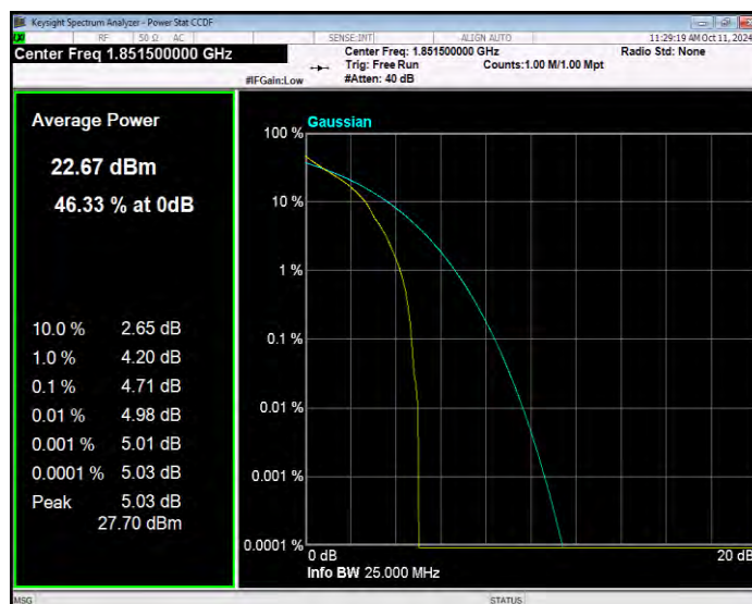
Band2 QPSK BW=3MHz Channel=18900 RB Size=1 Position=#0
