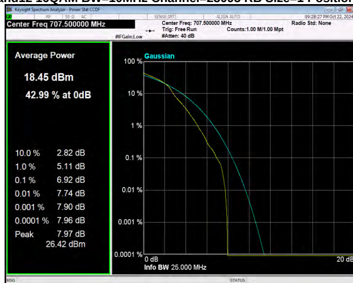
Band12 16QAM BW=10MHz Channel=23130 RB Size=1 Position=#0
