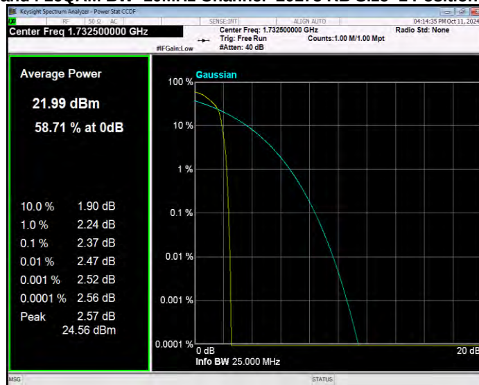
Band4 16QAM BW=10MHz Channel=20350 RB Size=1 Position=#0
