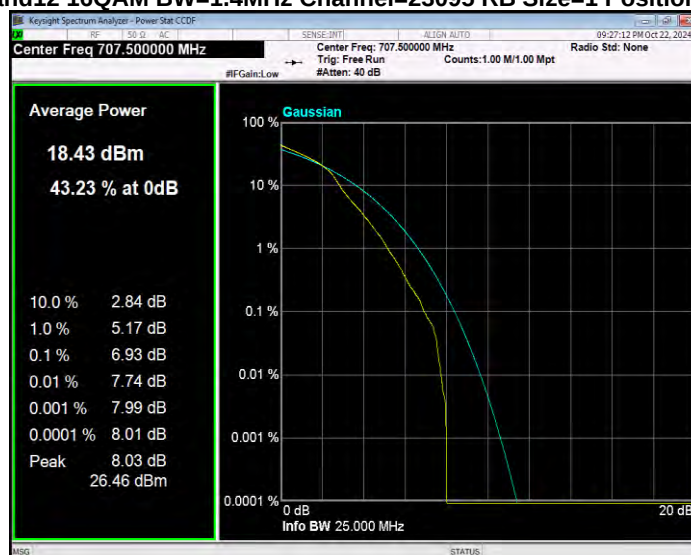
Band12 16QAM BW=1.4MHz Channel=23173 RB Size=1 Position=#0
