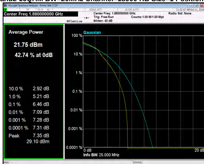
Band2 16QAM BW=20MHz Channel=19100 RB Size=1 Position=#0
