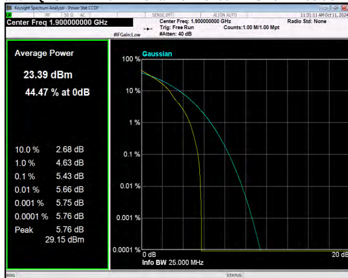
Band2 QPSK BW=3MHz Channel=18615 RB Size=1 Position=#0
