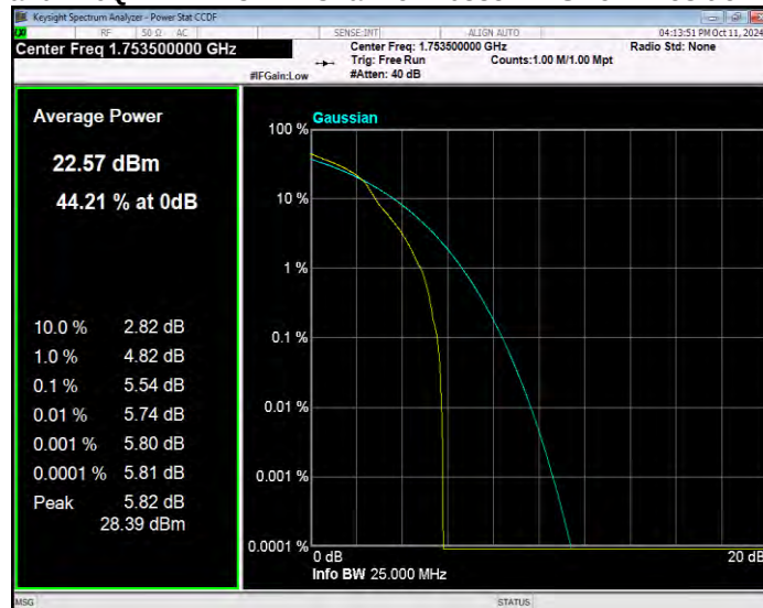
Band4 16QAM BW=5MHz Channel=19975 RB Size=1 Position=#0
