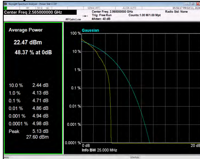
Band7 QPSK BW=15MHz Channel=20825 RB Size=1 Position=#0
