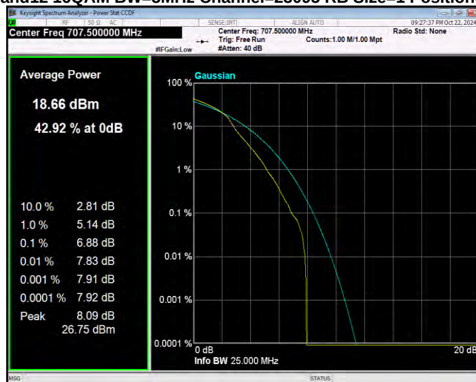
Band12 16QAM BW=3MHz Channel=23165 RB Size=1 Position=#0
