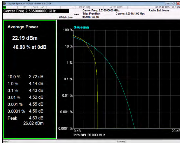
Band7 16QAM BW=5MHz Channel=21425 RB Size=1 Position=#0
