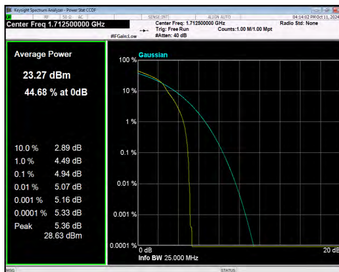
Band4 16QAM BW=5MHz Channel=20175 RB Size=1 Position=#0
