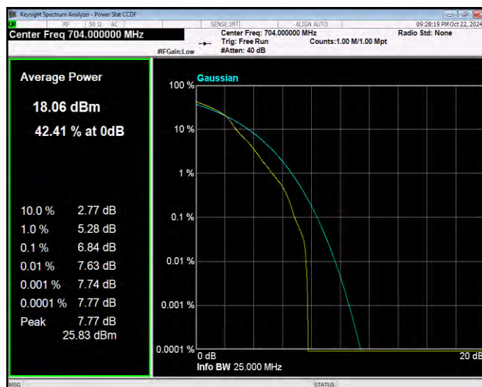
Band12 16QAM BW=10MHz Channel=23095 RB Size=1 Position=#0
