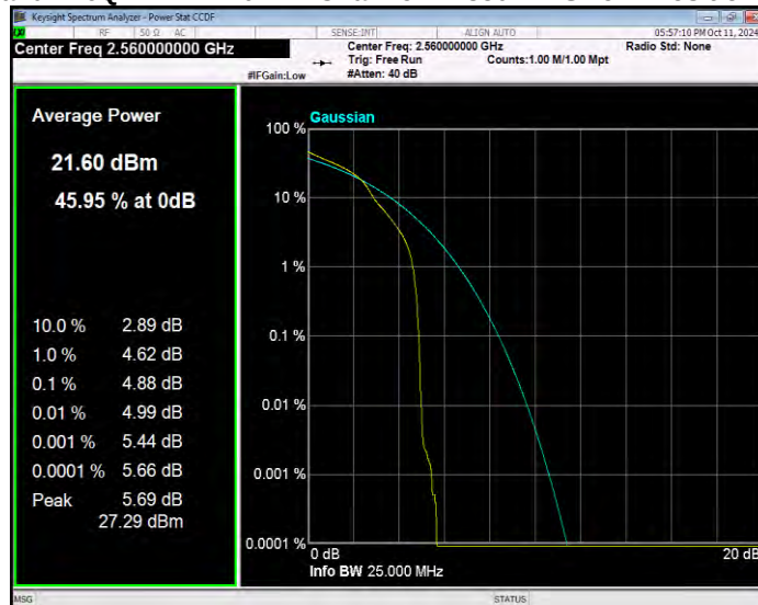
Band7 16QAM BW=5MHz Channel=20775 RB Size=1 Position=#0
