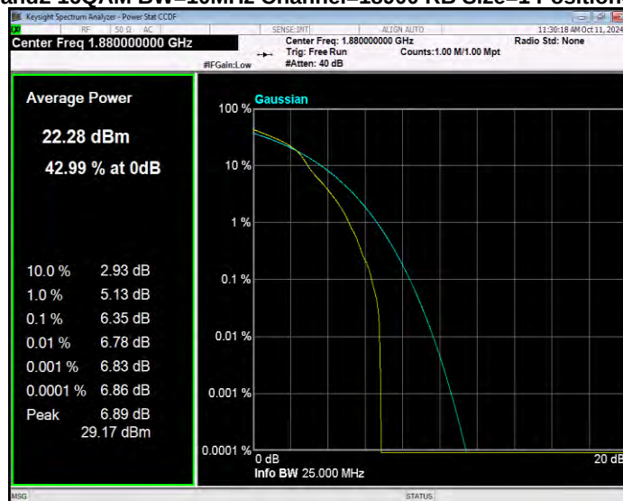
Band2 16QAM BW=10MHz Channel=19150 RB Size=1 Position=#0
