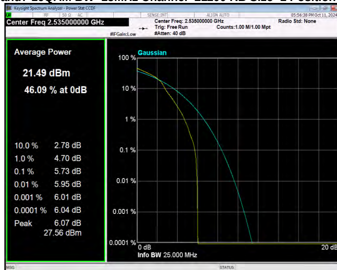
Band7 16QAM BW=15MHz Channel=21375 RB Size=1 Position=#0
