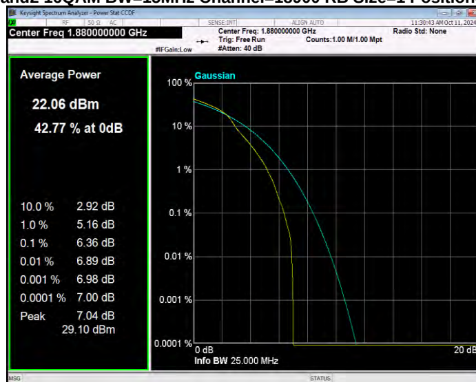
Band2 16QAM BW=15MHz Channel=19125 RB Size=1 Position=#0
