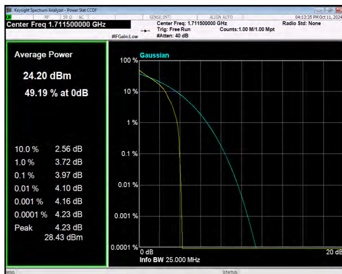
Band4 QPSK BW=3MHz Channel=20175 RB Size=1 Position=#0
