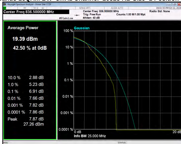
Band5 16QAM BW=3MHz Channel=20635 RB Size=1 Position=#0
