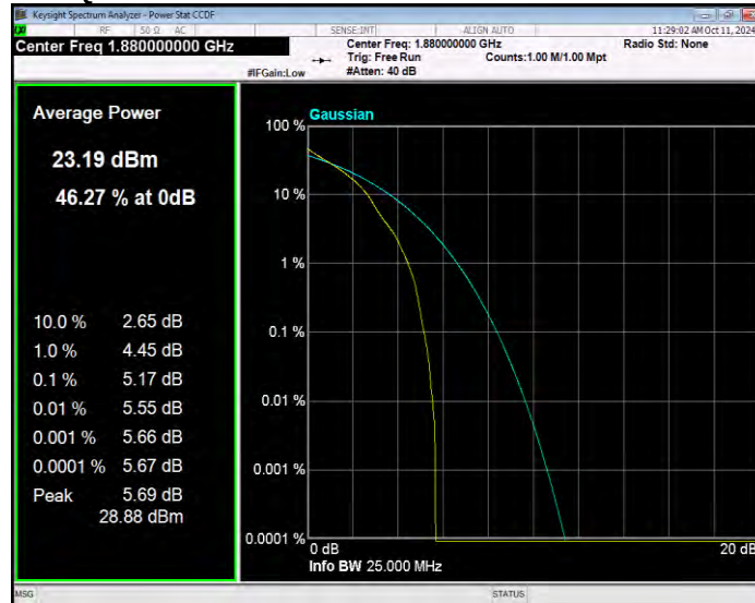
Band2 QPSK BW=1.4MHz Channel=19193 RB Size=1 Position=#0
