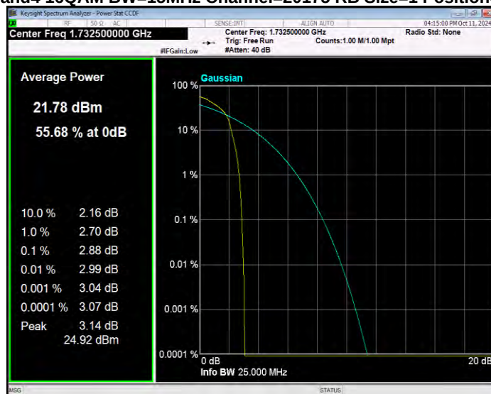
Band4 16QAM BW=15MHz Channel=20325 RB Size=1 Position=#0
