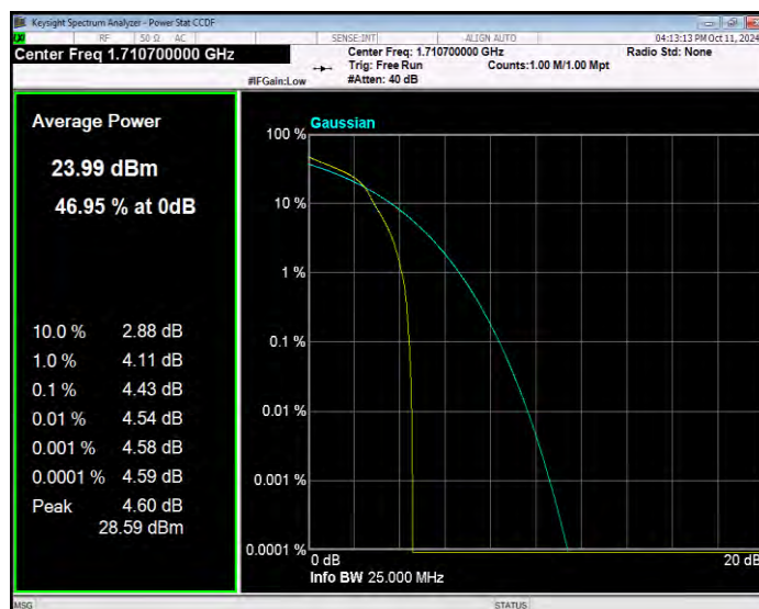
Band4 16QAM BW=1.4MHz Channel=20175 RB Size=1 Position=#0
