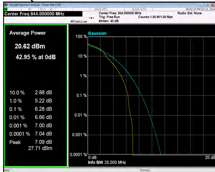
Band5 16QAM BW=3MHz Channel=20415 RB Size=1 Position=#0
