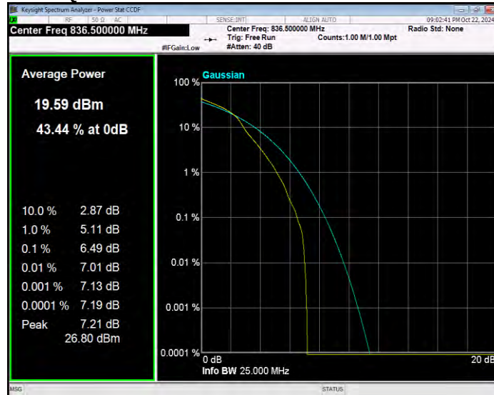
Band5 16QAM BW=10MHz Channel=20600 RB Size=1 Position=#0
