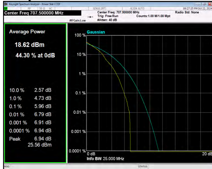
Band12 QPSK BW=3MHz Channel=23165 RB Size=1 Position=#0
