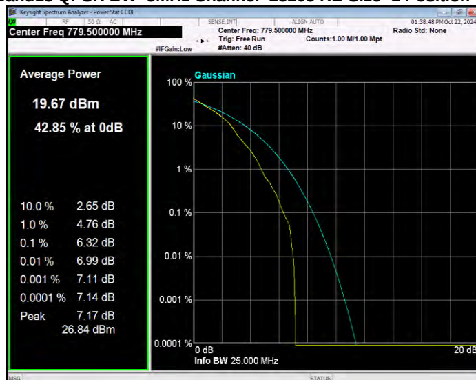
Band13 QPSK BW=5MHz Channel=23230 RB Size=1 Position=#0
