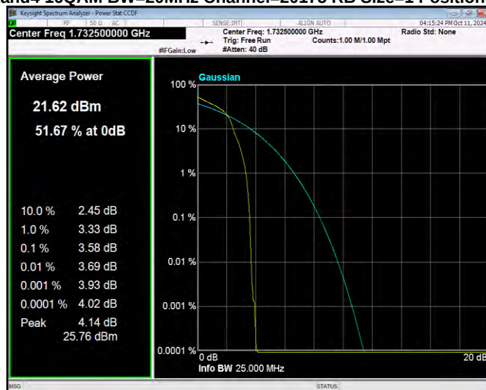
Band4 16QAM BW=20MHz Channel=20300 RB Size=1 Position=#0
