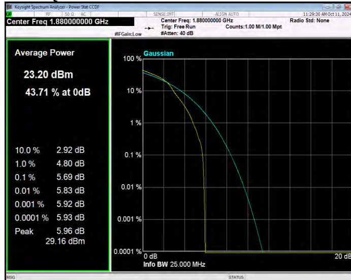
Band2 16QAM BW=3MHz Channel=19185 RB Size=1 Position=#0
