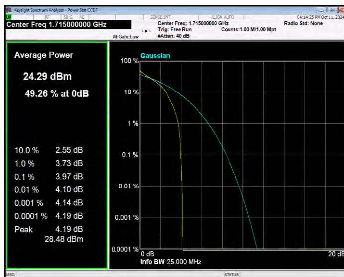
Band4 QPSK BW=10MHz Channel=20175 RB Size=1 Position=#0
