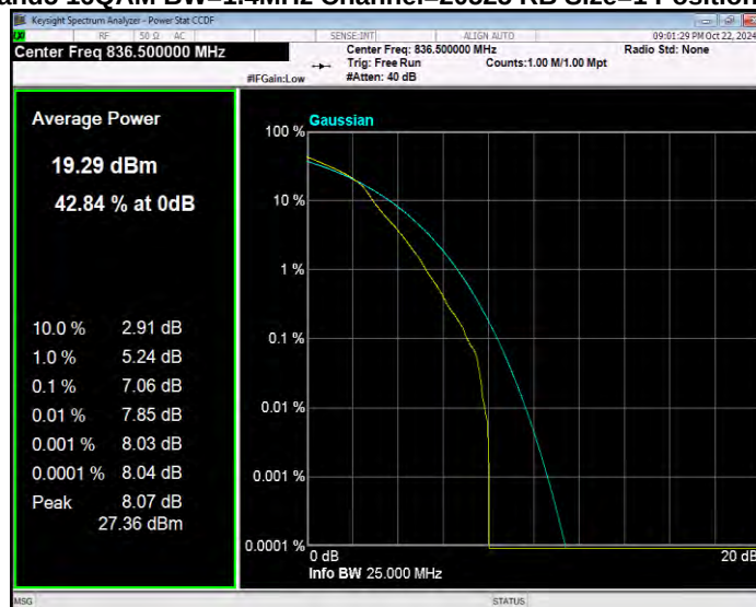
Band5 16QAM BW=1.4MHz Channel=20643 RB Size=1 Position=#0
