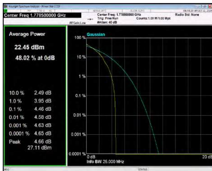
Band66 QPSK BW=5MHz Channel=131997 RB Size=1 Position=#0
