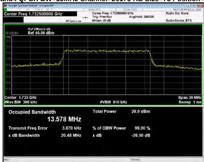
Band4 QPSK BW=15MHz Channel=20325 RB Size=75 Position=#0
