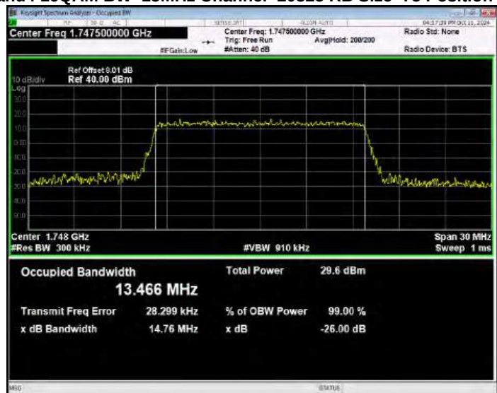
Band4 16QAM BW=20MHz Channel=20050 RB Size=100 Position=#0
