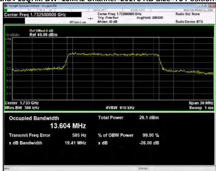
Band4 16QAM BW=15MHz Channel=20325 RB Size=75 Position=#0
