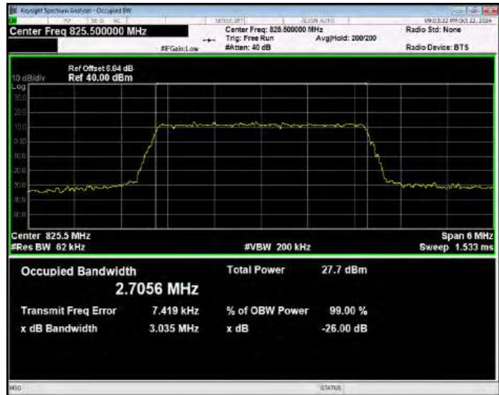
Band5 QPSK BW=3MHz Channel=20525 RB Size=15 Position=#0
