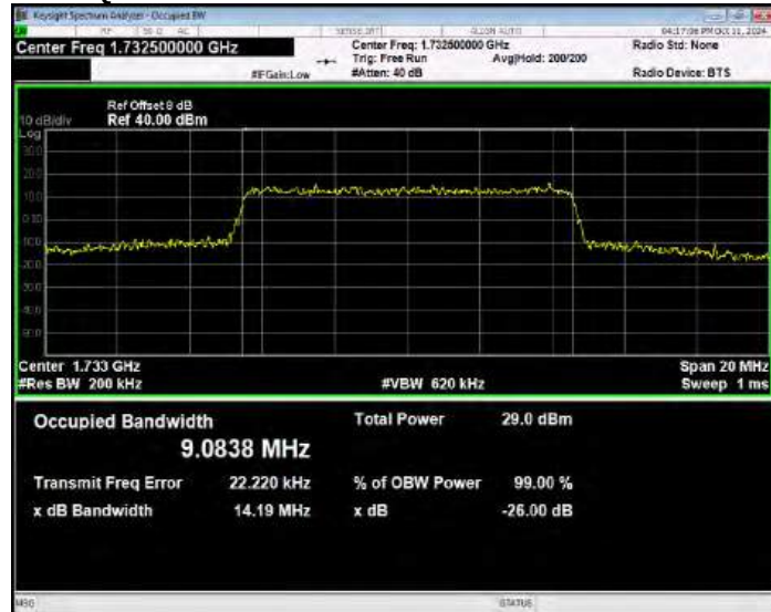
Band4 16QAM BW=10MHz Channel=20350 RB Size=50 Position=#0
