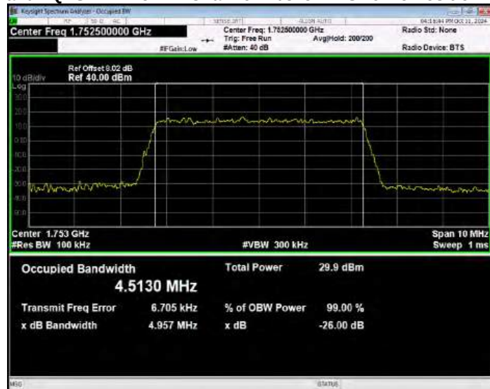
Band5 16QAM BW=1.4MHz Channel=20407 RB Size=6 Position=#0
