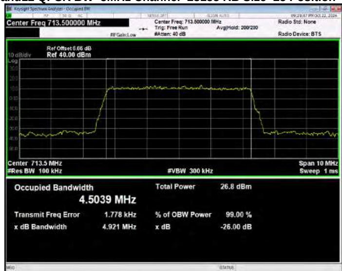
Band13 16QAM BW=10MHz Channel=23230 RB Size=50 Position=#0
