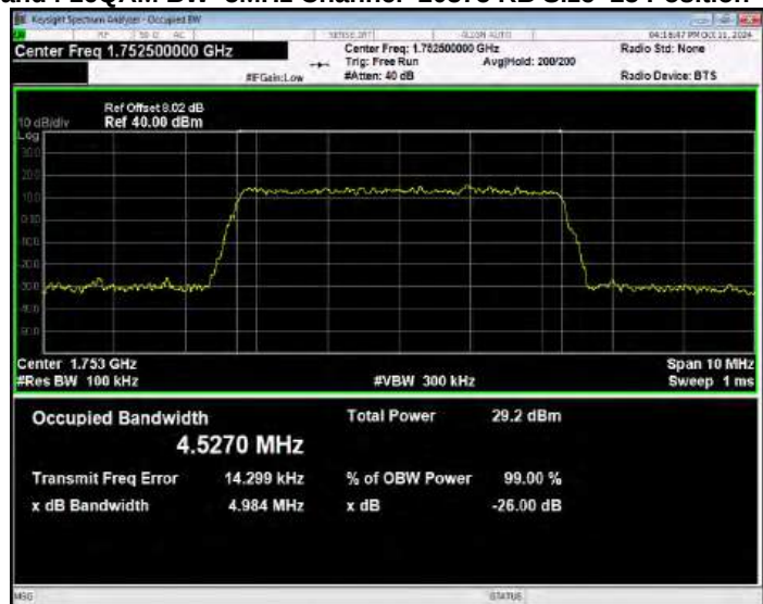
Band4 QPSK BW=1.4MHz Channel=19957 RB Size=6 Position=#0
