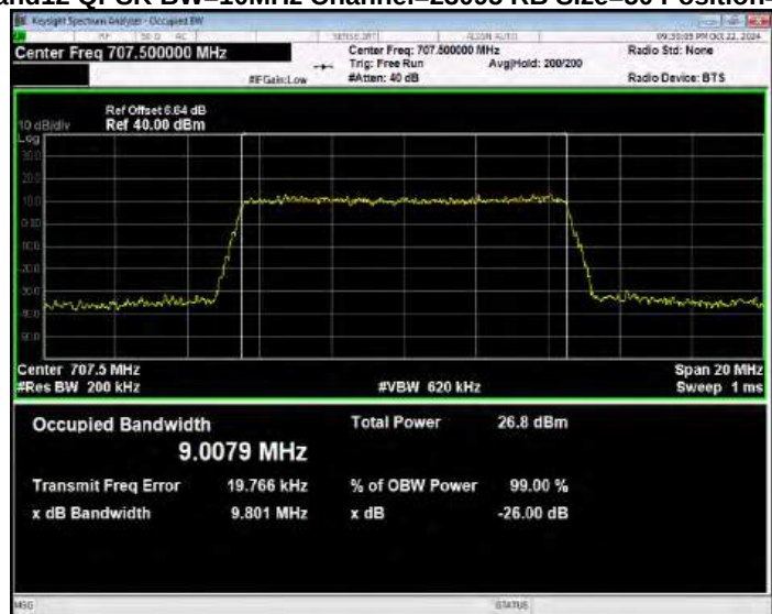
Band12 QPSK BW=10MHz Channel=23130 RB Size=50 Position=#0
