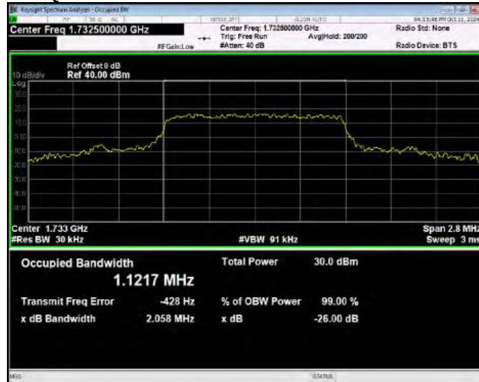
Band4 QPSK BW=1.4MHz Channel=20393 RB Size=6 Position=#0
