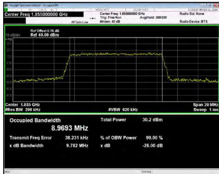
Band2 QPSK BW=10MHz Channel=18900 RB Size=50 Position=#0
