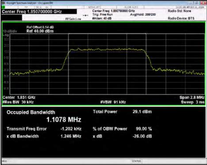
Band2 16QAM BW=1.4MHz Channel=18900 RB Size=6 Position=#0
