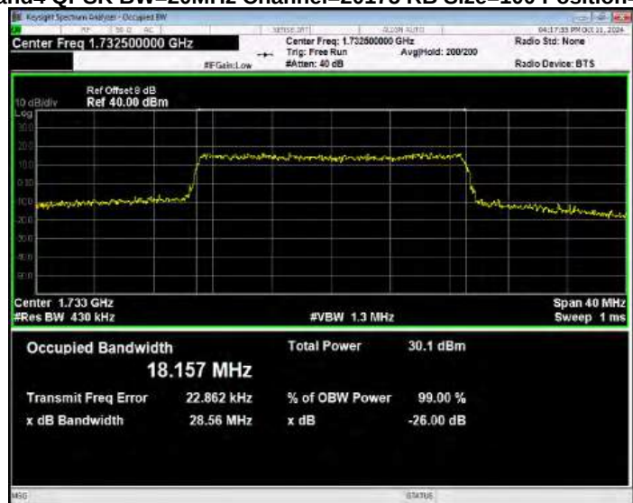
Band4 QPSK BW=20MHz Channel=20300 RB Size=100 Position=#0
