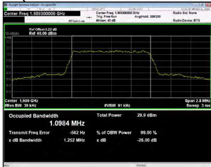
Band2 QPSK BW=10MHz Channel=18650 RB Size=50 Position=#0
