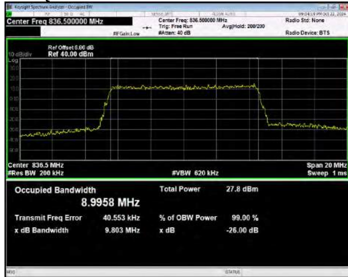
Band5 16QAM BW=10MHz Channel=20600 RB Size=50 Position=#0
