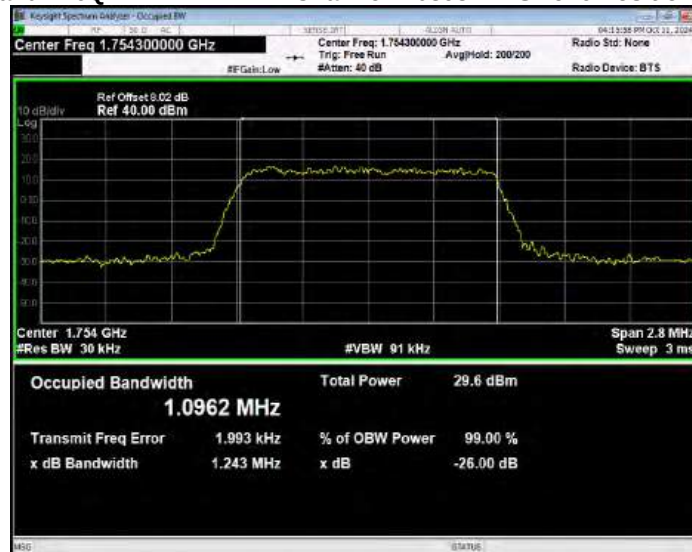
Band4 16QAM BW=10MHz Channel=20000 RB Size=50 Position=#0
