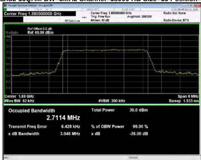
Band2 16QAM BW=3MHz Channel=19185 RB Size=15 Position=#0
