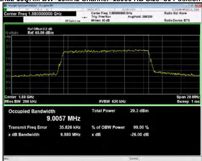
Band2 16QAM BW=10MHz Channel=19150 RB Size=50 Position=#0
