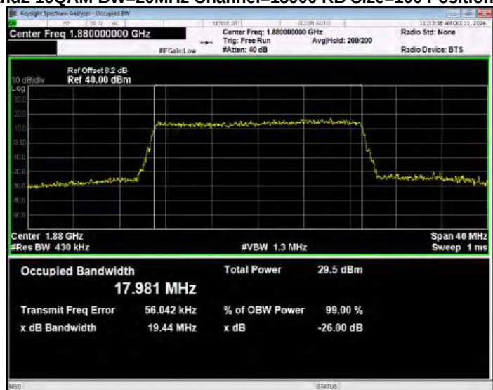
Band2 16QAM BW=20MHz Channel=19100 RB Size=100 Position=#0
