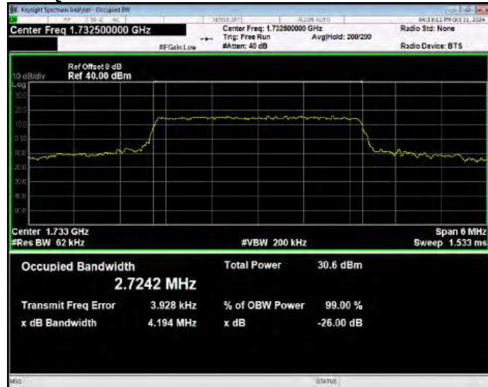
Band4 QPSK BW=3MHz Channel=20385 RB Size=15 Position=#0
