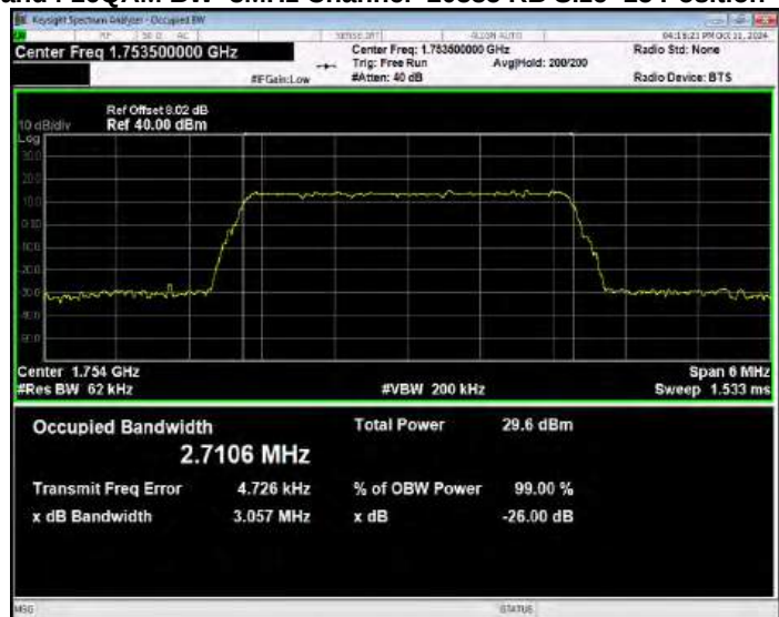
Band4 16QAM BW=5MHz Channel=19975 RB Size=25 Position=#0
