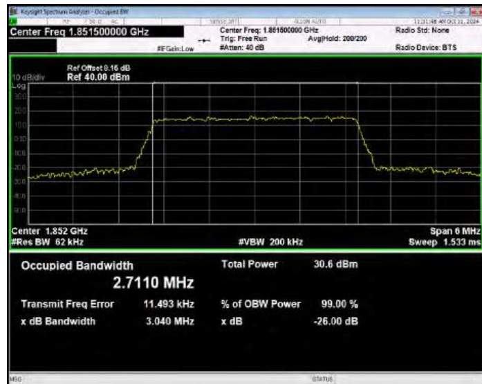
Band2 QPSK BW=3MHz Channel=18900 RB Size=15 Position=#0
