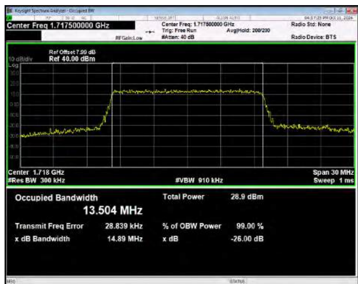
Band4 16QAM BW=15MHz Channel=20175 RB Size=75 Position=#0
