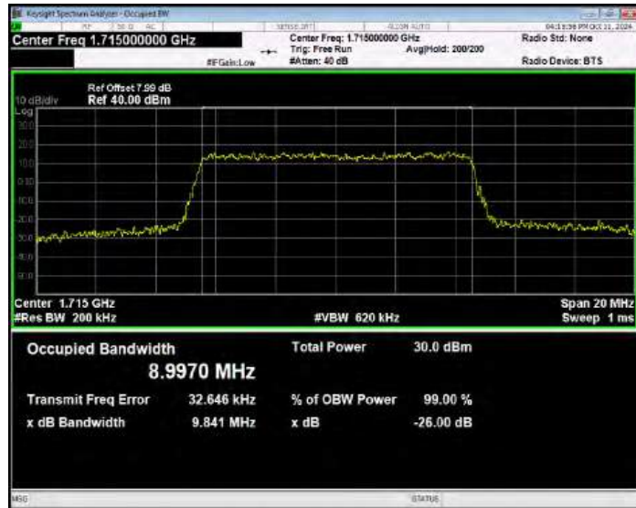
Band4 QPSK BW=10MHz Channel=20175 RB Size=50 Position=#0
