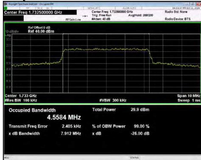
Band4 QPSK BW=5MHz Channel=20375 RB Size=25 Position=#0
