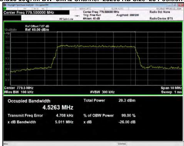
Band13 16QAM BW=5MHz Channel=23230 RB Size=25 Position=#0
