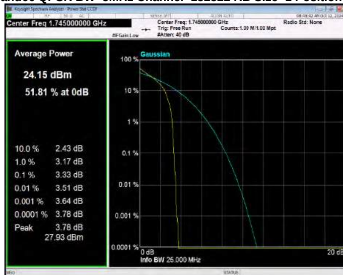
Band66 QPSK BW=5MHz Channel=132647 RB Size=1 Position=#0
