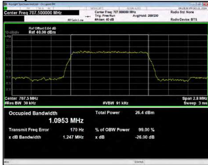
Band12 QPSK BW=1.4MHz Channel=23173 RB Size=6 Position=#0
