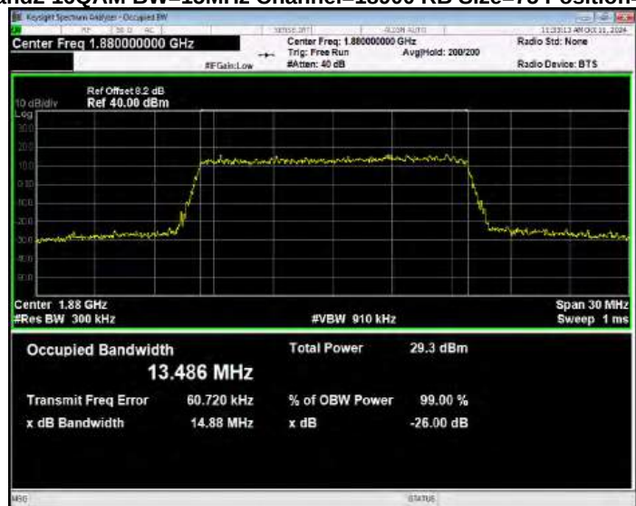
Band2 16QAM BW=15MHz Channel=19125 RB Size=75 Position=#0
