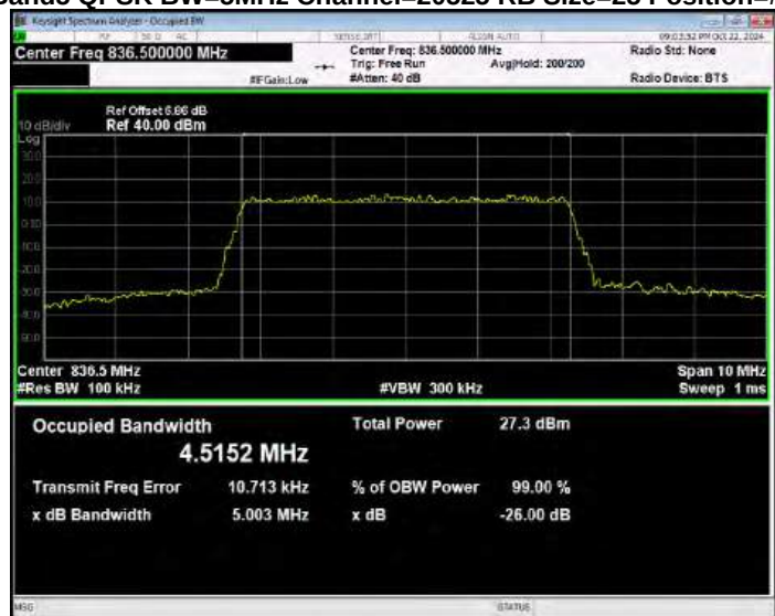
Band5 QPSK BW=5MHz Channel=20625 RB Size=25 Position=#0
