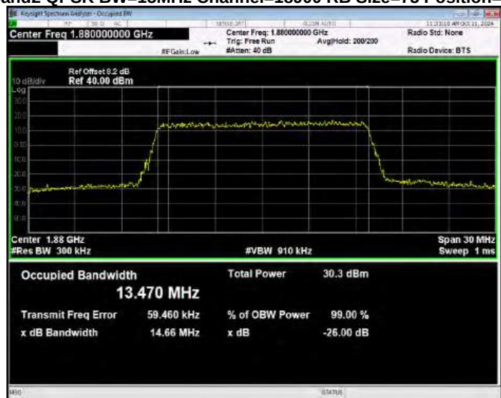
Band2 QPSK BW=15MHz Channel=19125 RB Size=75 Position=#0
