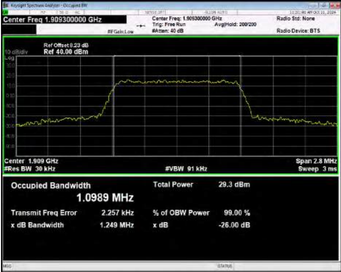
Band2 16QAM BW=10MHz Channel=18650 RB Size=50 Position=#0
