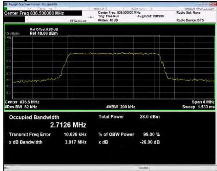
Band5 QPSK BW=3MHz Channel=20635 RB Size=15 Position=#0
