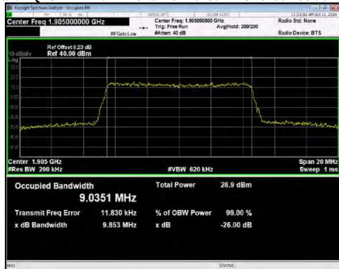
Band2 QPSK BW=15MHz Channel=18675 RB Size=75 Position=#0
