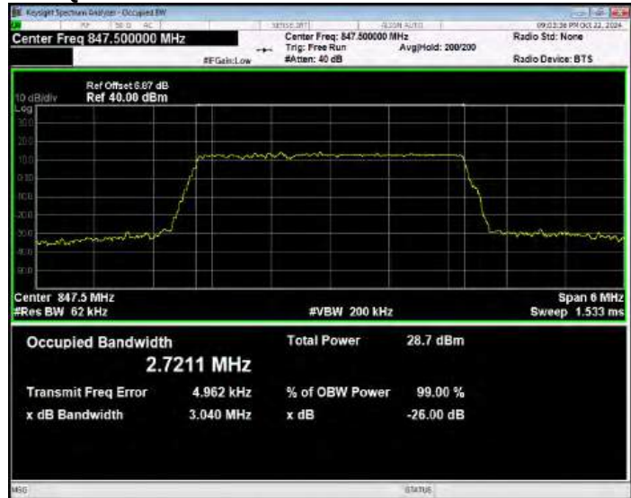
Band5 QPSK BW=5MHz Channel=20425 RB Size=25 Position=#0
