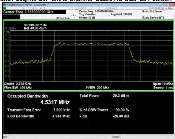
Band7 16QAM BW=5MHz Channel=21425 RB Size=25 Position=#0
