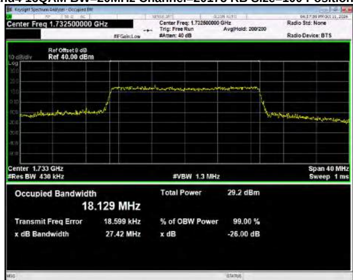
Band4 16QAM BW=20MHz Channel=20300 RB Size=100 Position=#0
