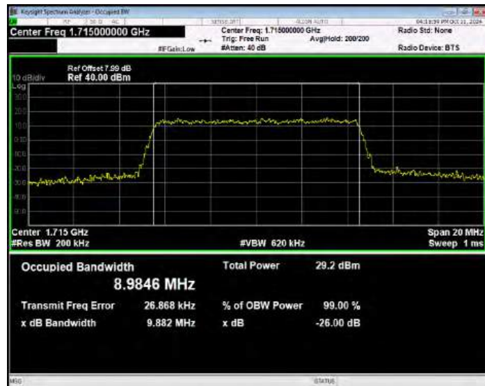
Band4 16QAM BW=10MHz Channel=20175 RB Size=50 Position=#0
