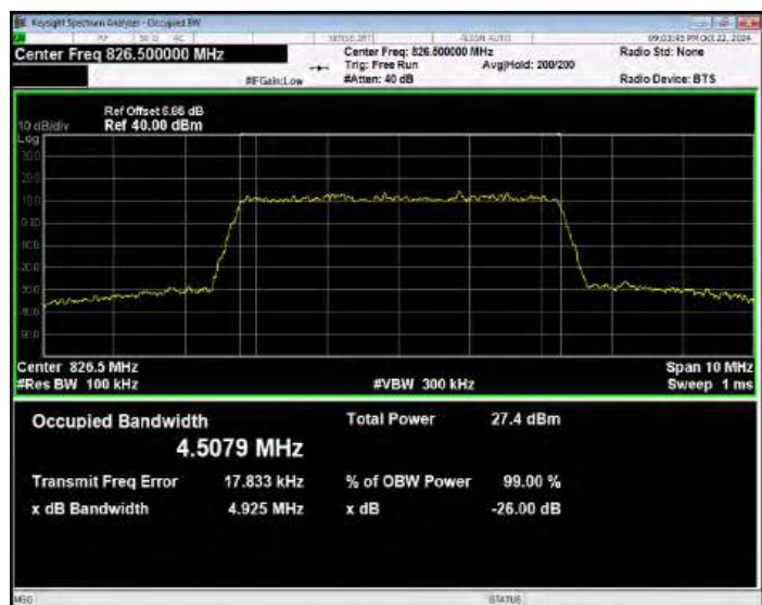
Band5 QPSK BW=5MHz Channel=20525 RB Size=25 Position=#0
