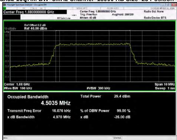
Band2 16QAM BW=5MHz Channel=19175 RB Size=25 Position=#0
