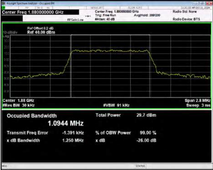
Band2 16QAM BW=1.4MHz Channel=19193 RB Size=6 Position=#0
