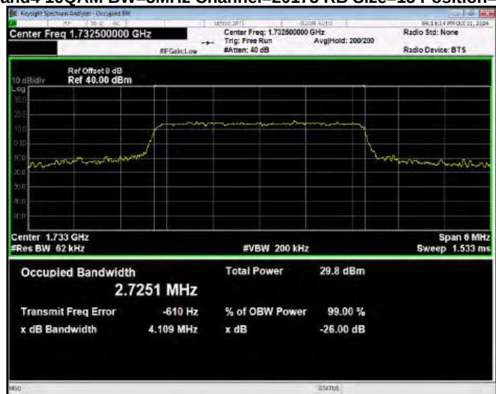
Band4 16QAM BW=3MHz Channel=20385 RB Size=15 Position=#0
