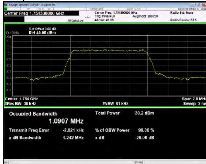
Band4 QPSK BW=10MHz Channel=20000 RB Size=50 Position=#0
