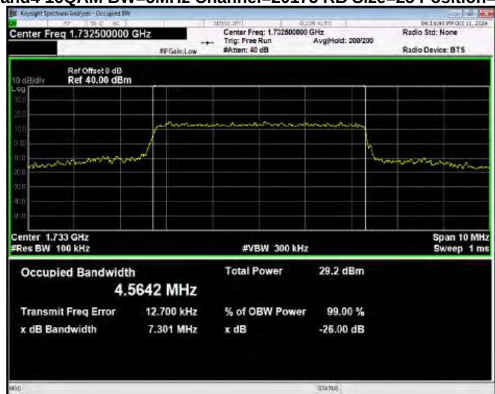
Band4 16QAM BW=5MHz Channel=20375 RB Size=25 Position=#0
