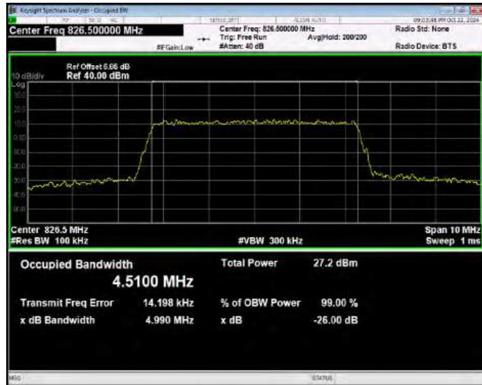
Band5 16QAM BW=5MHz Channel=20525 RB Size=25 Position=#0
