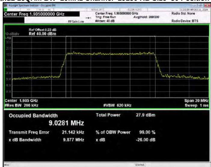
Band2 16QAM BW=15MHz Channel=18675 RB Size=75 Position=#0
