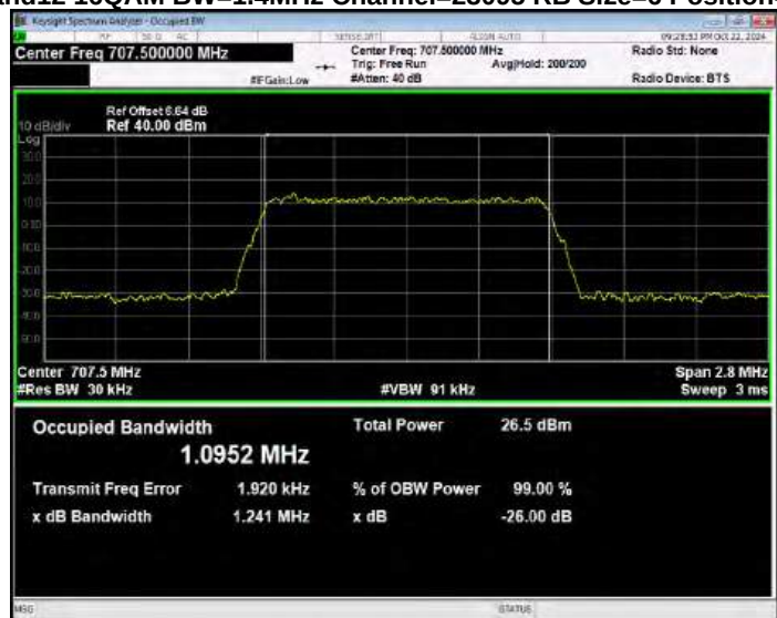
Band12 16QAM BW=1.4MHz Channel=23173 RB Size=6 Position=#0
