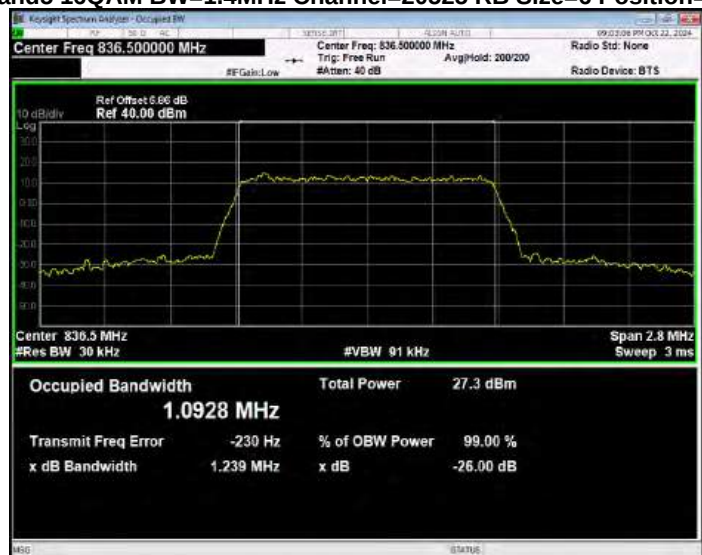
Band5 16QAM BW=1.4MHz Channel=20643 RB Size=6 Position=#0
