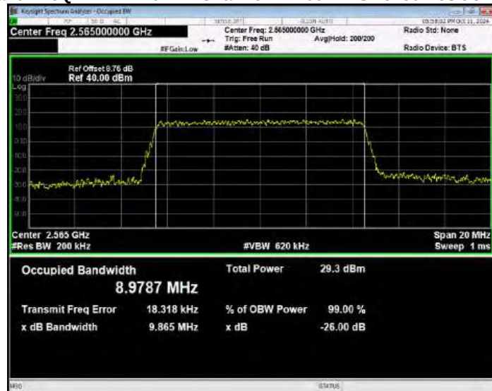
Band7 16QAM BW=15MHz Channel=20825 RB Size=75 Position=#0
