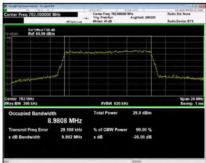
Band13 16QAM BW=5MHz Channel=23205 RB Size=25 Position=#0
