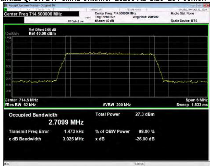
Band12 QPSK BW=5MHz Channel=23035 RB Size=25 Position=#0
