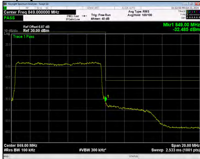
Band26(824-849) 16QAM BW=15MHz Channel=26865 RB Size=1 Position=#0 Extended
