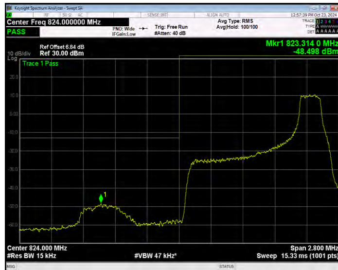
Band26(824-849) QPSK BW=1.4MHz Channel=26797 RB Size=6 Position=#0 Extended
