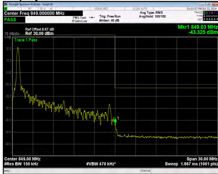
Band26(824-849) 16QAM BW=15MHz Channel=26965 RB Size=1 Position=#Max Extended
