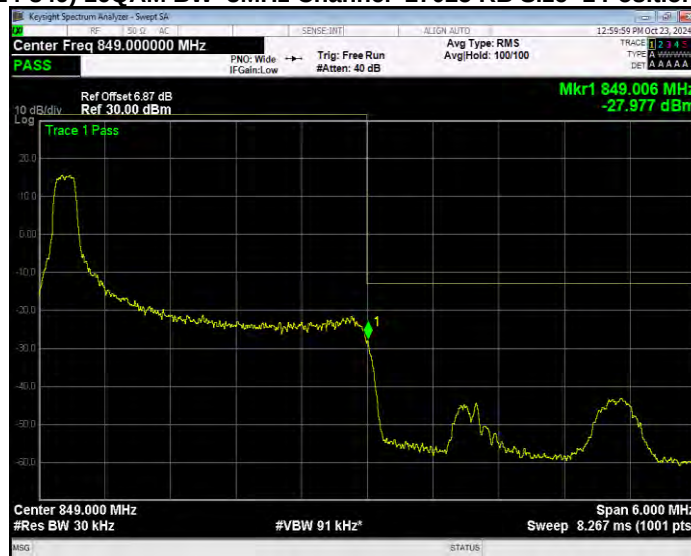
Band26(824-849) 16QAM BW=3MHz Channel=27025 RB Size=1 Position=#Max Extended
