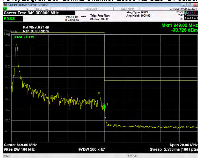
Band26(824-849) 16QAM BW=10MHz Channel=26990 RB Size=1 Position=#Max Extended
