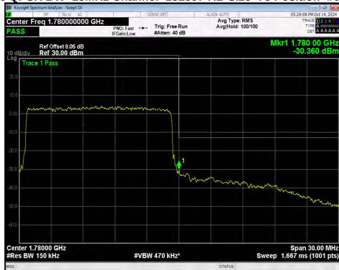
Band66 QPSK BW=20MHz Channel=132072 RB Size=1 Position=#0 Extended
