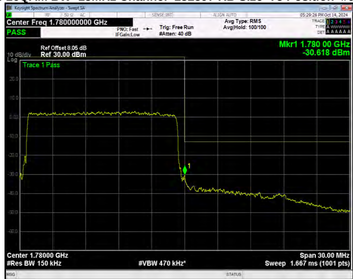
Band66 16QAM BW=20MHz Channel=132072 RB Size=1 Position=#0 Extended
