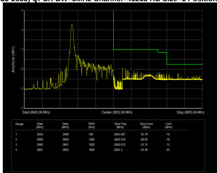
Band41(2535-2655) QPSK BW=5MHz Channel=41215 RB Size=1 Position=#Max Extended
