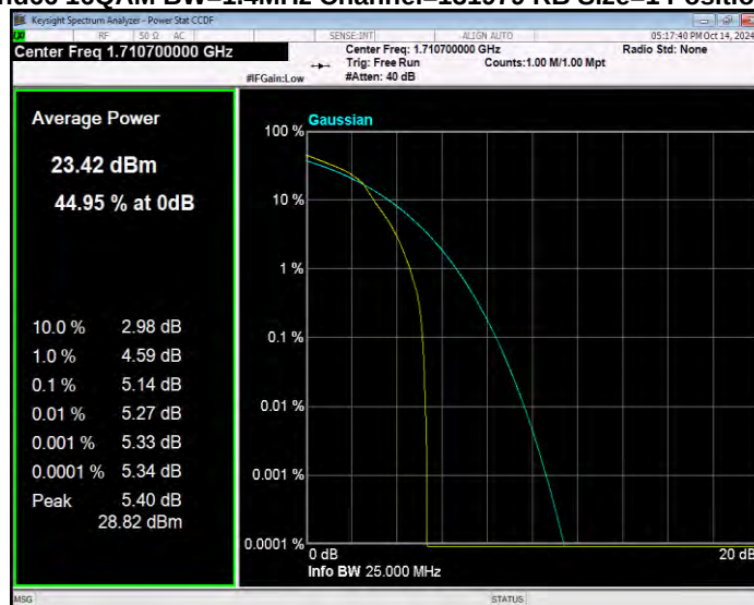
Band66 16QAM BW=1.4MHz Channel=132322 RB Size=1 Position=#0
