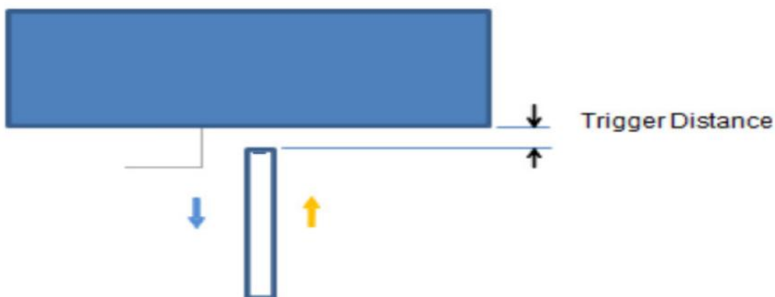
Picture: Proximity sensor triggering distances assessment (bottom/Top)
