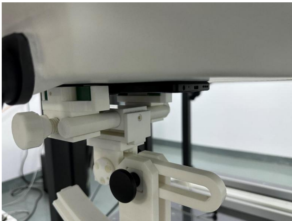
Body Front side (separation distance is 0mm)
