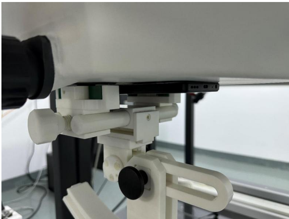
Body Back side (separation distance is 0mm)
