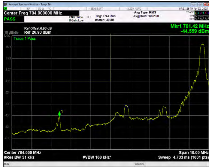
Band17 QPSK BW=5MHz Channel=23755 RB Size=25 Position=#0 Normal
