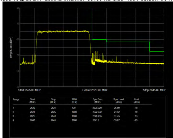
Band38 16QAM BW=5MHz Channel=37775 RB Size=1 Position=#Max Normal
