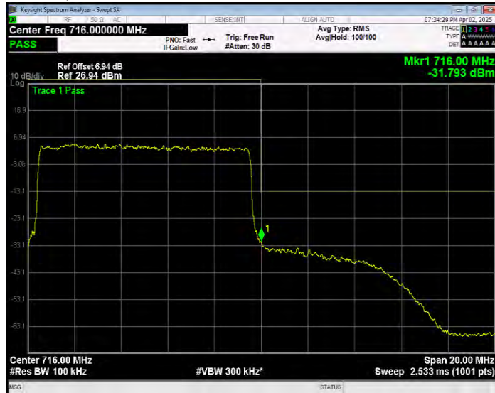
Band17 16QAM BW=10MHz Channel=23800 RB Size=50 Position=#0 Extended
