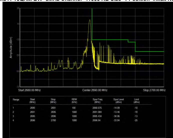
Band41 QPSK BW=10MHz Channel=39700 RB Size=1 Position=#0 Normal
