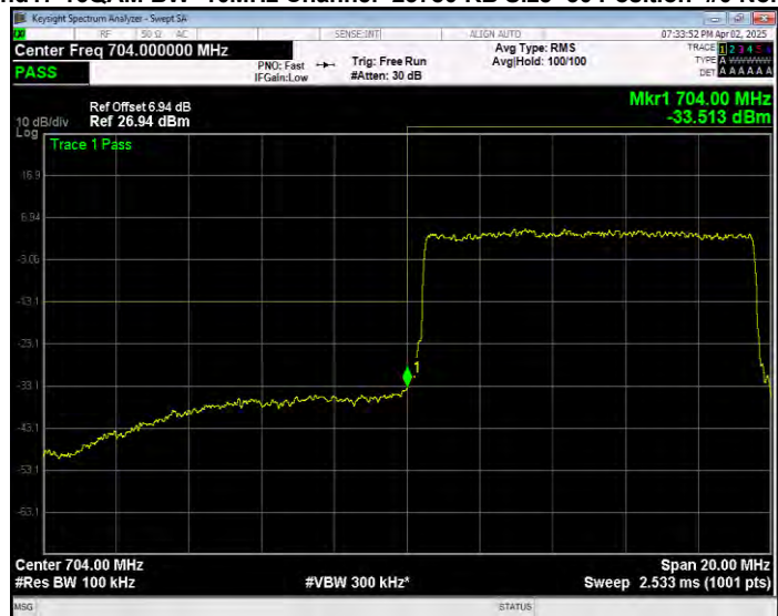
Band17 16QAM BW=10MHz Channel=23800 RB Size=1 Position=#0 Normal
