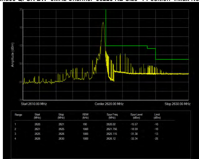
Band38 QPSK BW=5MHz Channel=38225 RB Size=25 Position=#0 Normal
