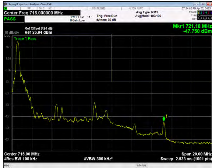
Band17 QPSK BW=10MHz Channel=23800 RB Size=1 Position=#Max Normal
