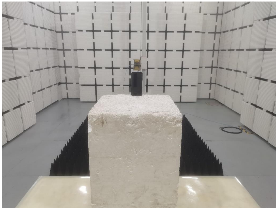
Set-up for Radiated Spurious Emission, Above 1GHz
