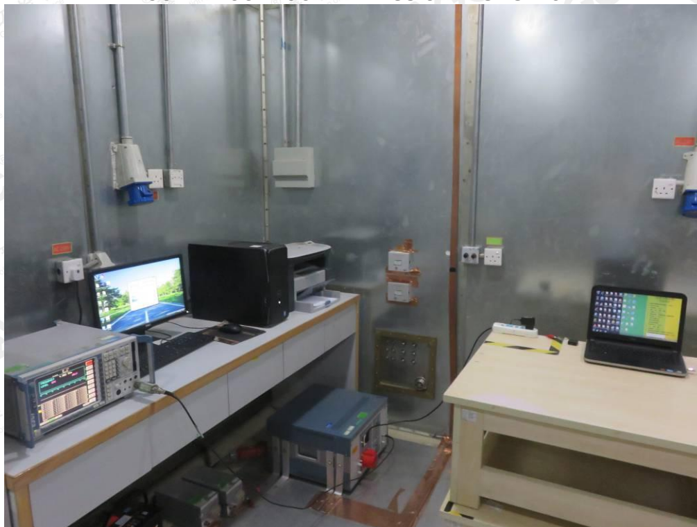
FCC RADIATED EMISSION TEST SETUP
