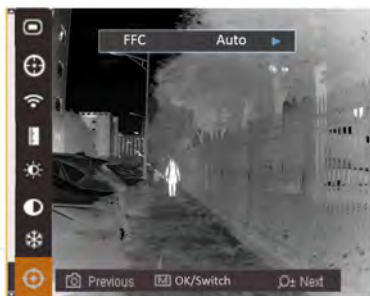
Figure 3-4 Flat Field Correction
