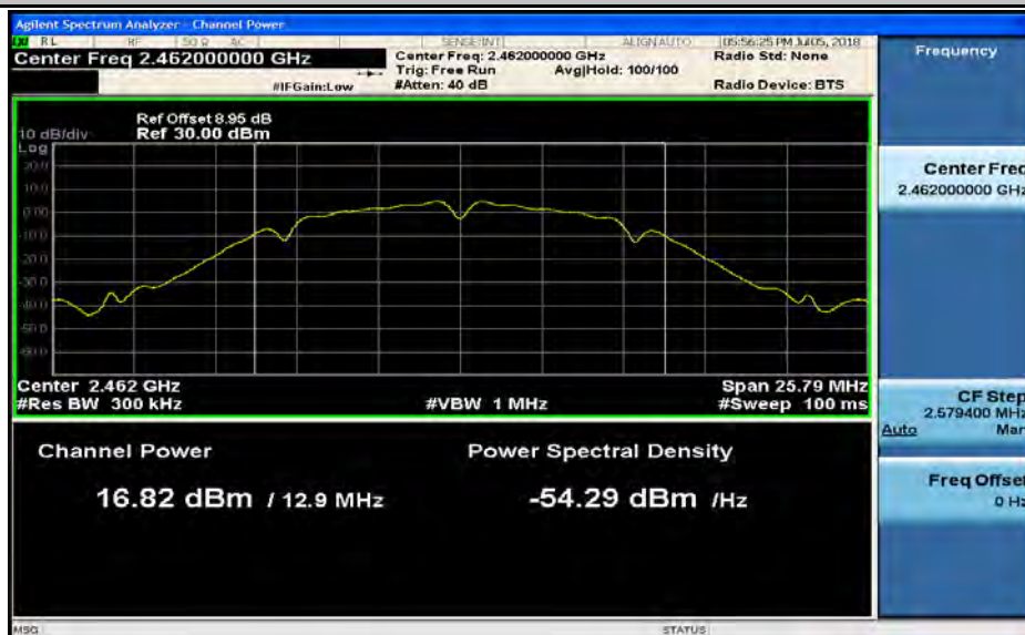
Maximum conducted (average) output power_11B_2462_Ant1
