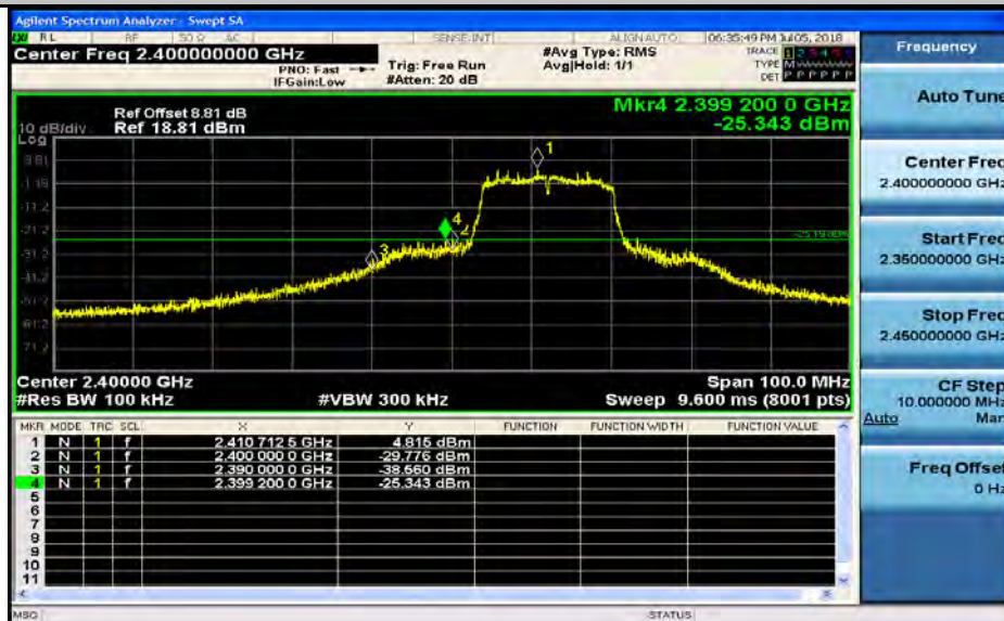
Band-edge for RF Conducted Emissions_11G_2412_Ant1
