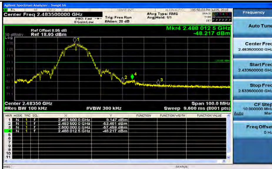
Band-edge for RF Conducted Emissions_11G_2412_Ant1
