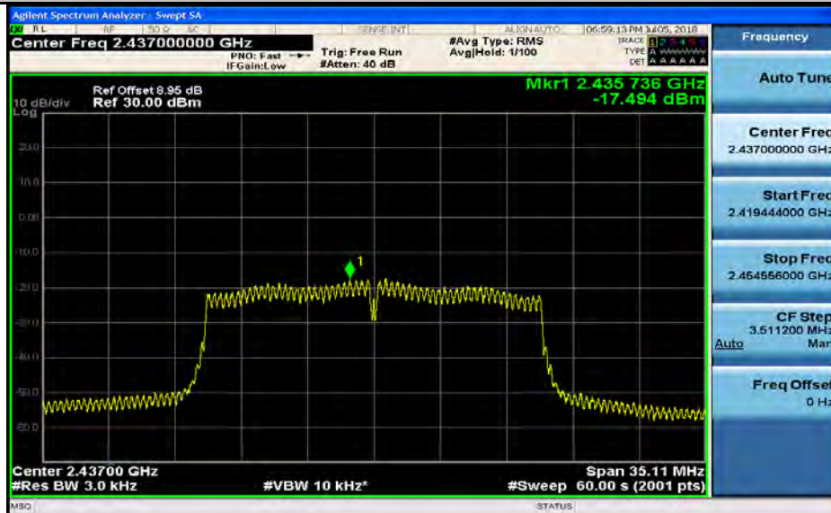
Maximum(average) power spectral density_11N20SISO_2462_Ant1
