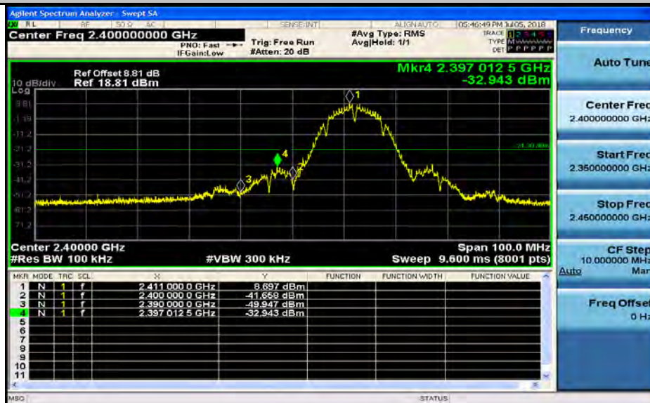
Band-edge for RF Conducted Emissions_11B_2462_Ant1
