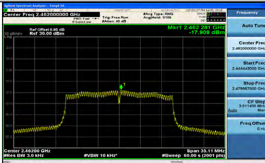
Maximum(average) power spectral density_11N20SISO_2462_Ant1
