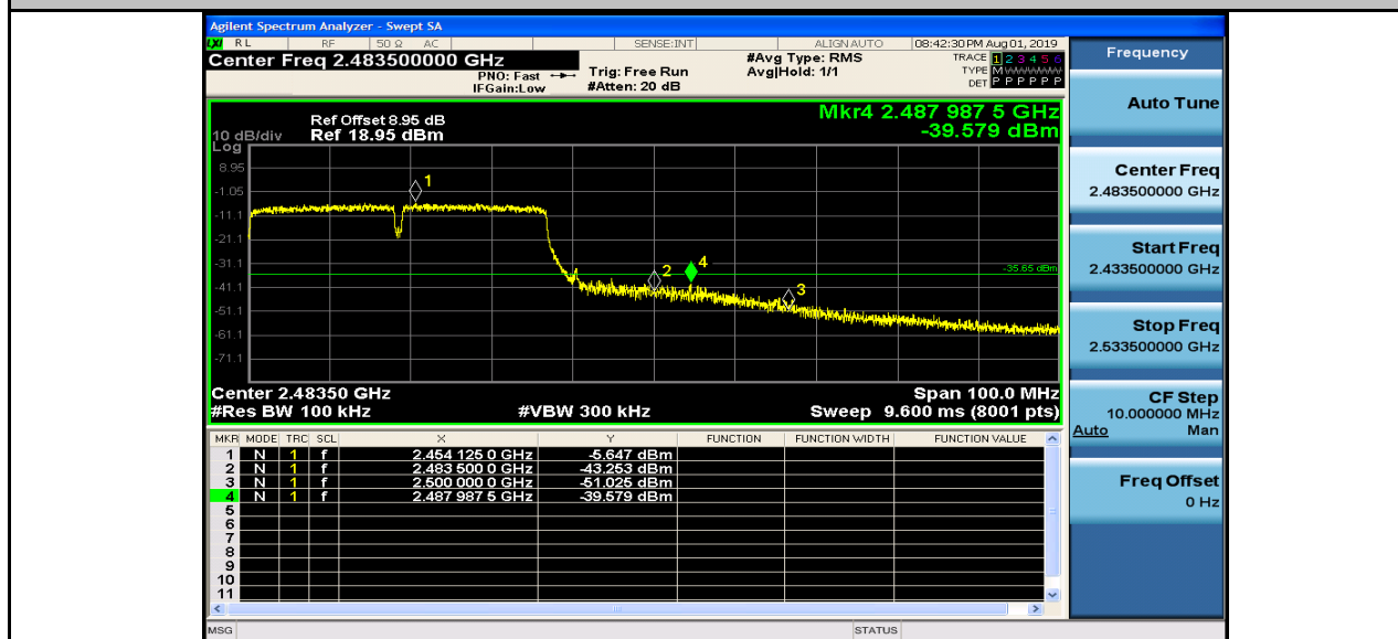
Band-edge for RF Conducted Emissions_11N40SISO_2452_Ant2
