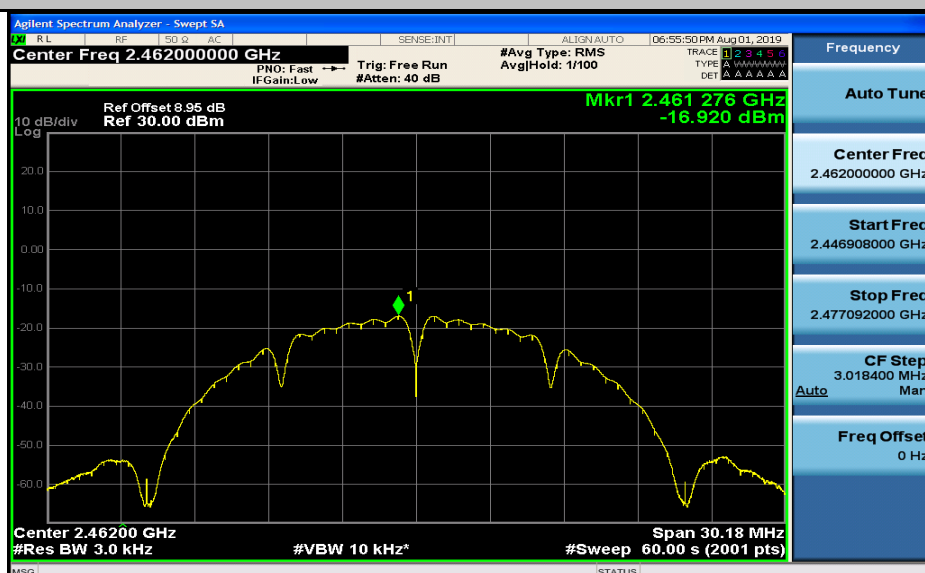
Maximum(average) power spectral density_11B_2462_Ant1
