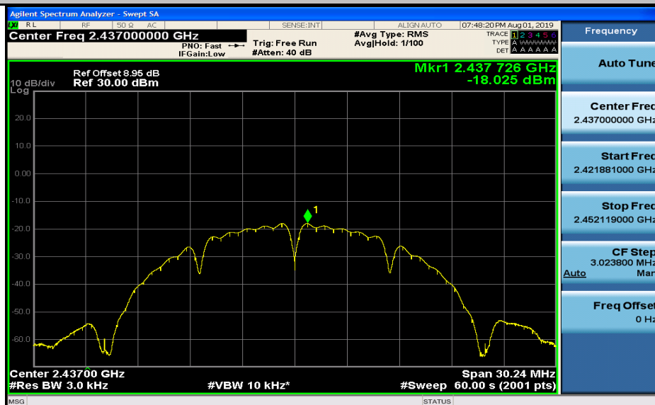
Maximum(average) power spectral density_11B_2462_Ant2
