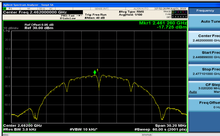
Maximum(average) power spectral density_11B_2462_Ant2
