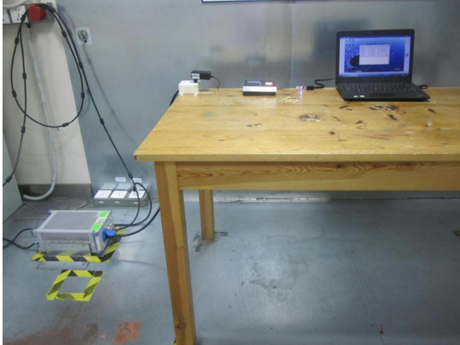
Photograph 1: Set-up for Conducted Emission on AC Mains
