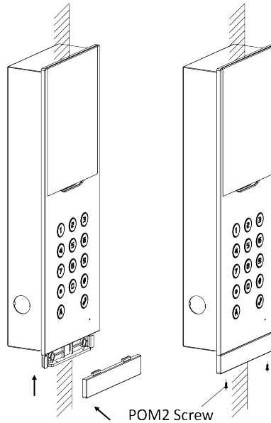
Figure 3-5 Fix the Door Station
