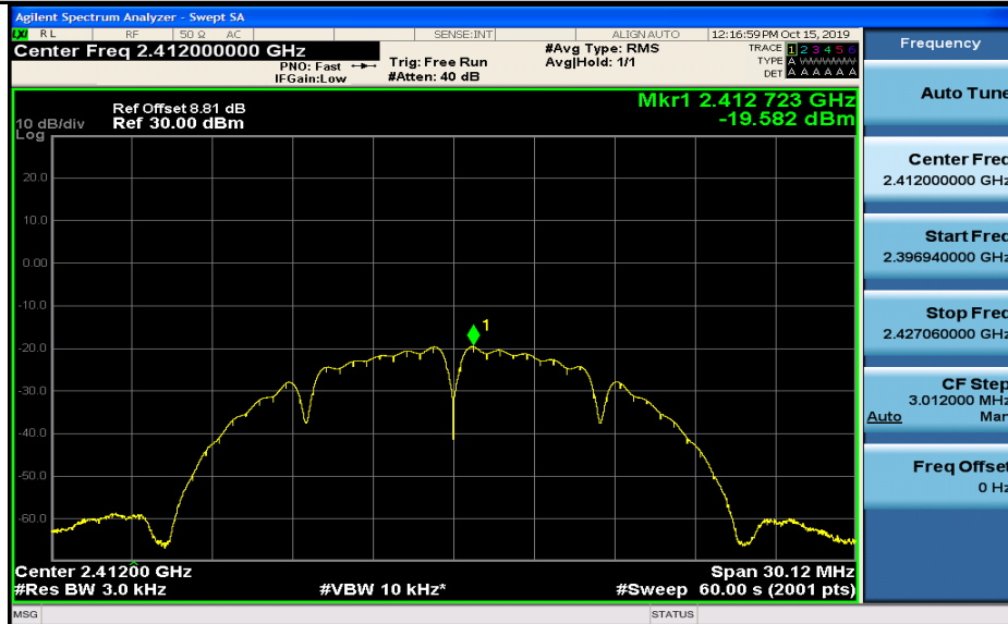
Maximum(average) power spectral density_11B_2437_Ant1
