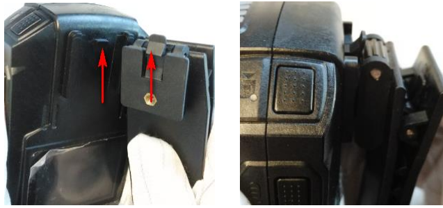
Figure 1. 5 Install Shoulder Clip
