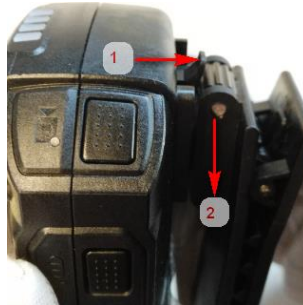
Figure 1. 6 Uninstall Shoulder Clip
