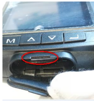
Figure 1. 4 Close the SIM Card
