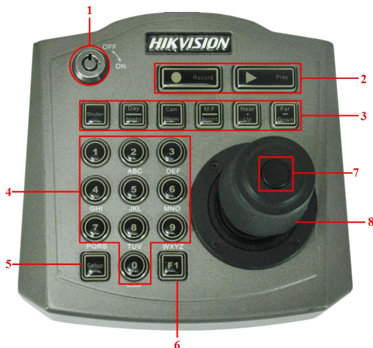
Figure 2-3 Manual Controller View
