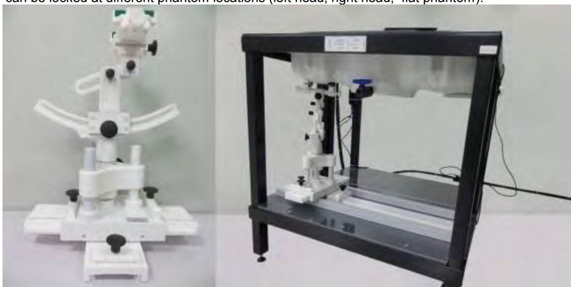
Device holder supplied by SATIMO
