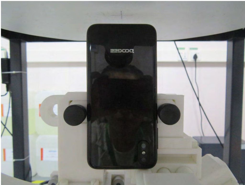
10mm body-worn Top Side Setup Photo (hotspot)
