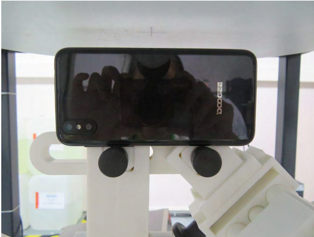
10mm body-worn Left Side Setup Photo(hotspot)
