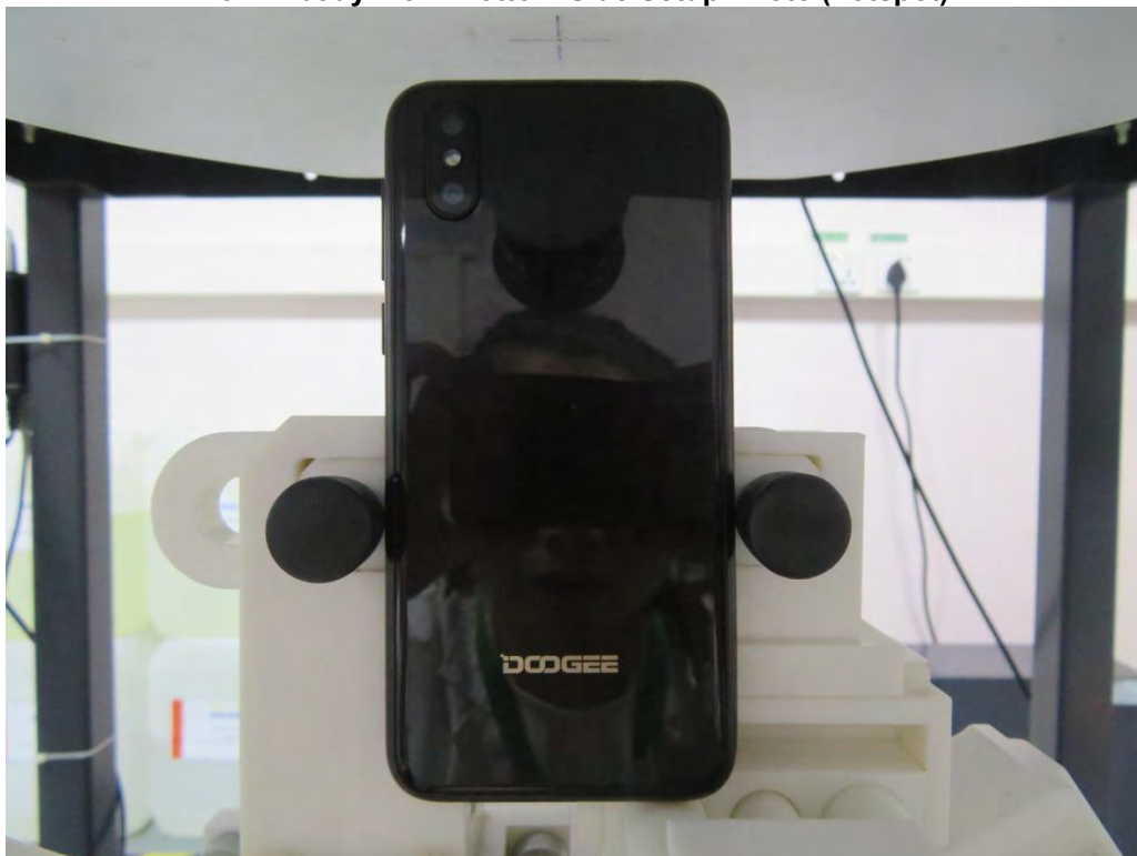
10mm body-worn Bottom Side Setup Photo (hotspot)
