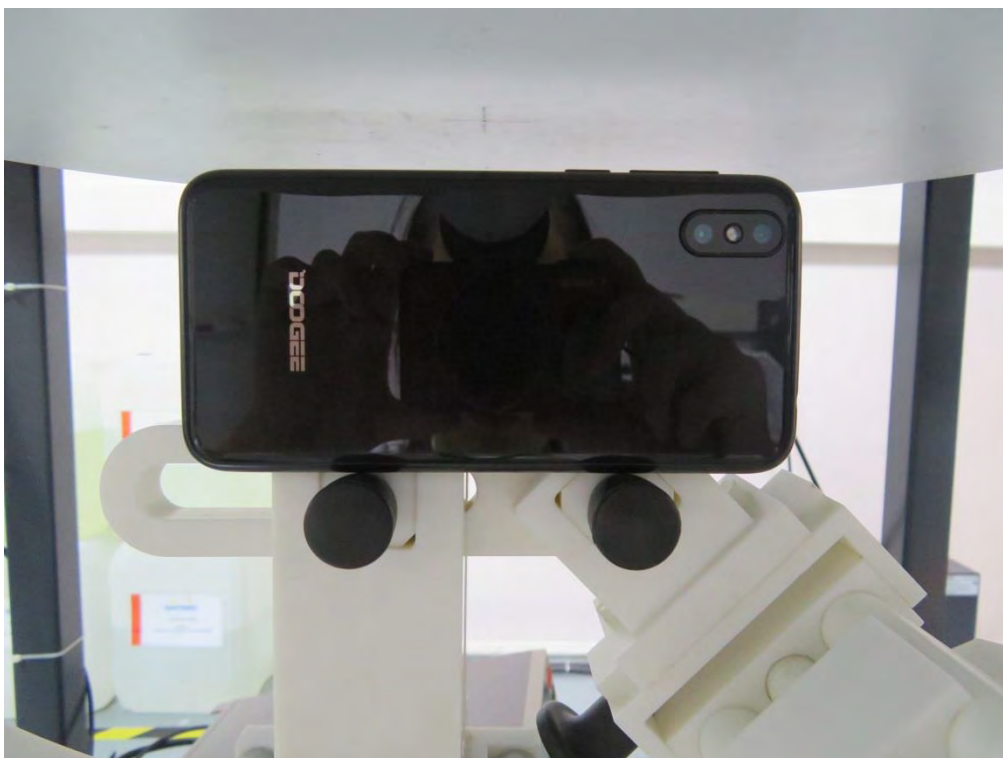
10mm body-worn Right Side Setup Photo (hotspot)
