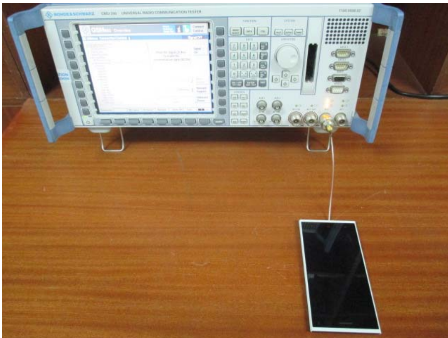
Photograph – 2G&3G Conducted Test Setup
