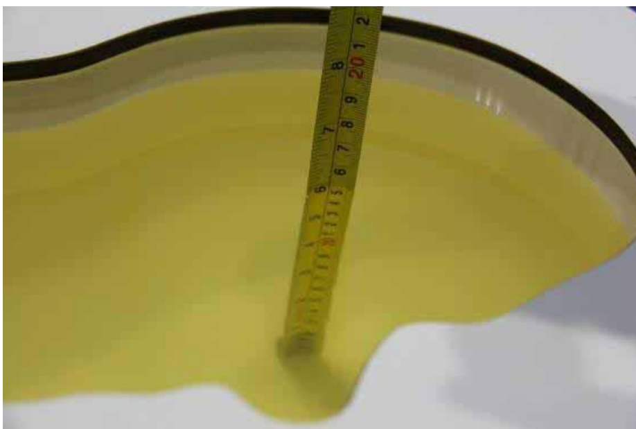
Liquid depth in the Head Phantom (1900 MHz) (depth>15cm)
