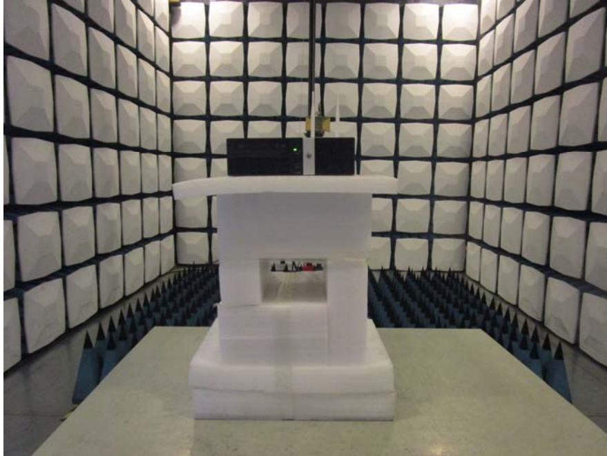
Radiated Emission View (Above 1GHz)
