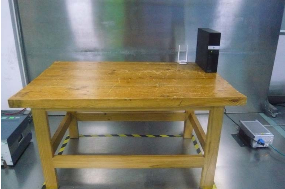
Conducted Emissions – Front View
