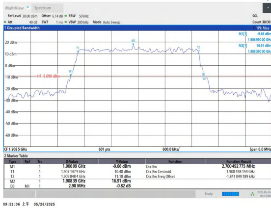
Band2-3MHz-QPSK-19185-15RB#0-PASS
