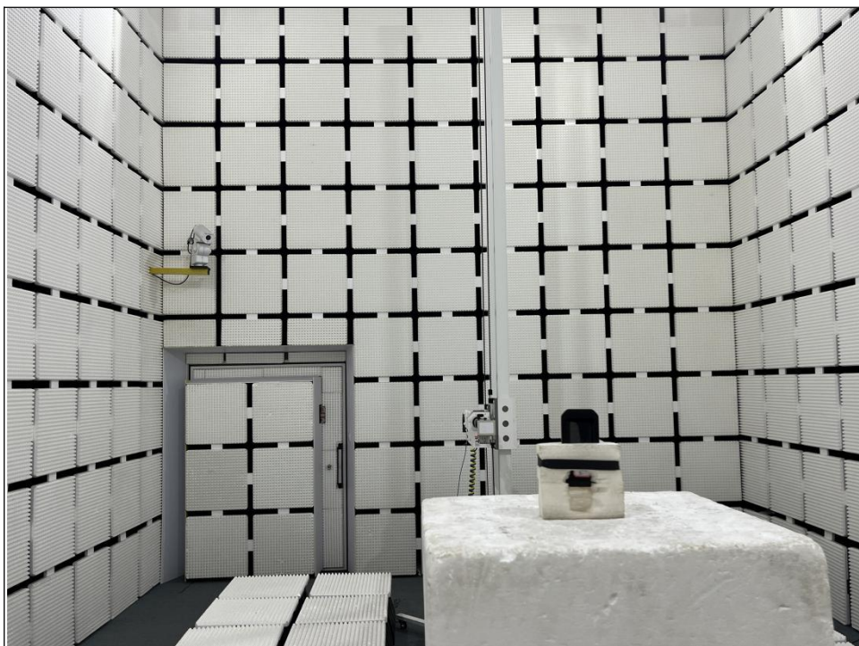
RADIATED EMISSION TEST (18GHz ~ 40GHz)
