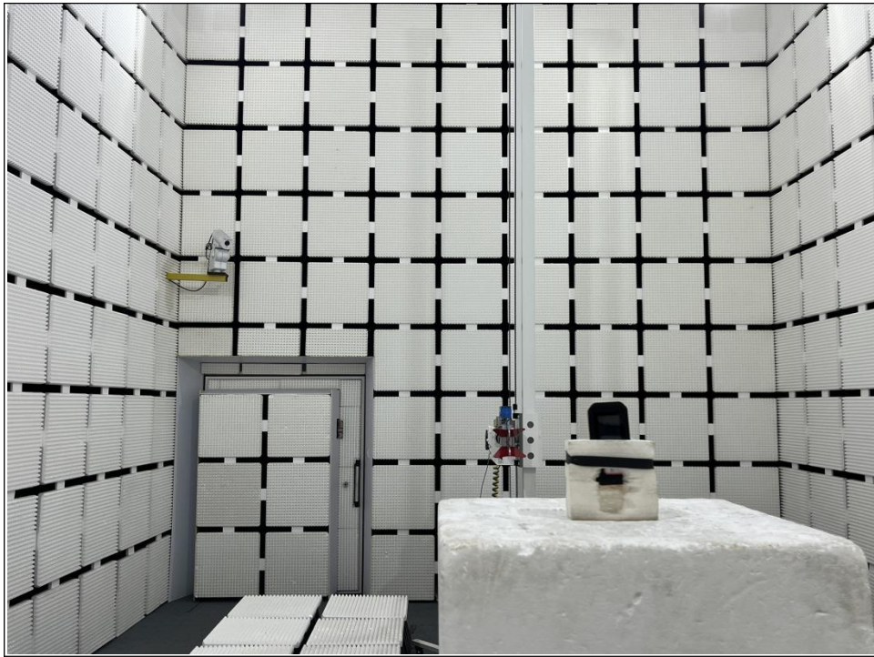
RADIATED EMISSION TEST (1GHz ~ 18GHz)
