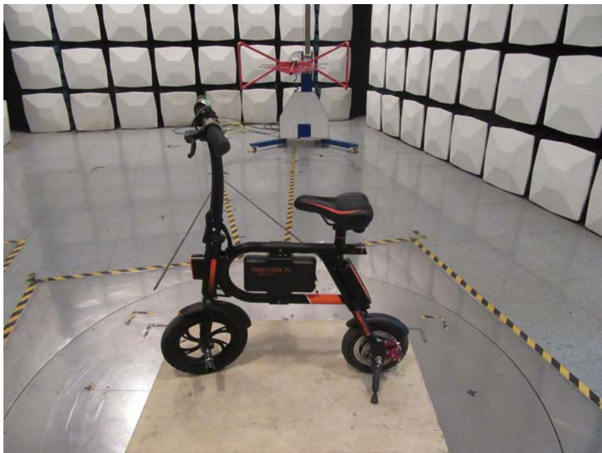
Radiated Emission View (Below 1GHz)
