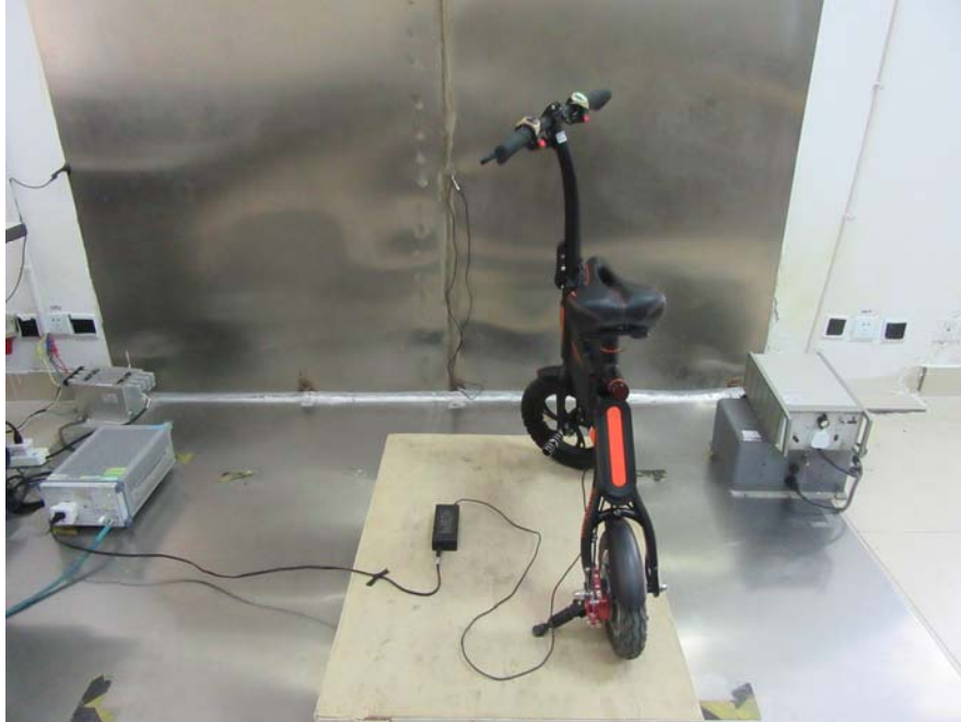
Conducted Emission View
