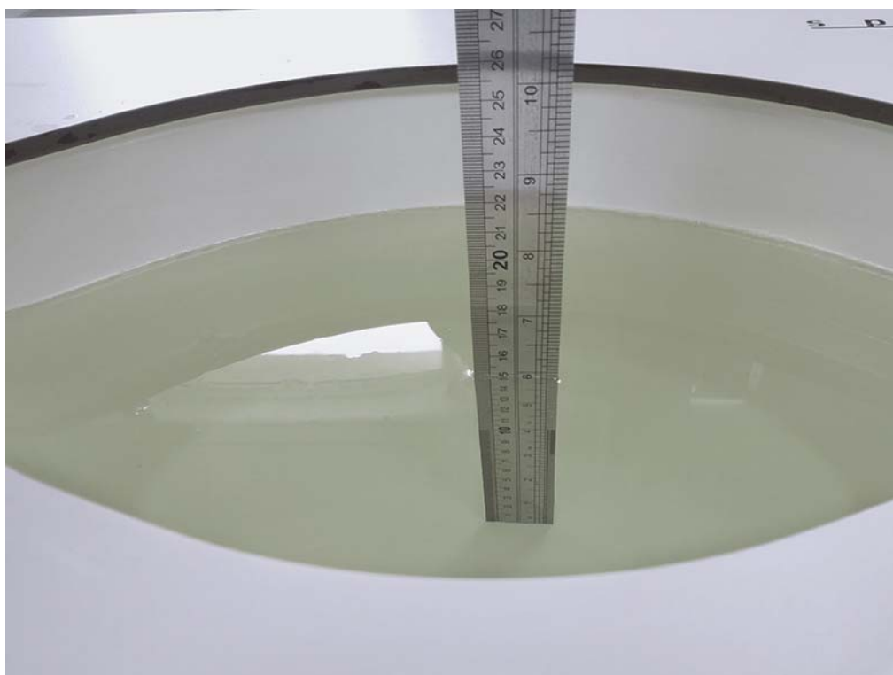
Liquid depth in the flat Phantom (2450 MHz, 15.1cm depth)
