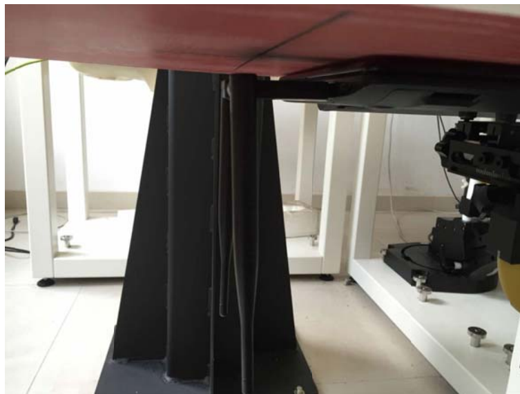
Test Position 1: 5 mm separation from the flat phantom for the bottom of the dangle at Horizontal-Up;
