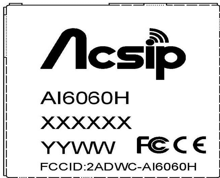
Figure 1 Standard Product Marking Diagram- TOP VIEW
